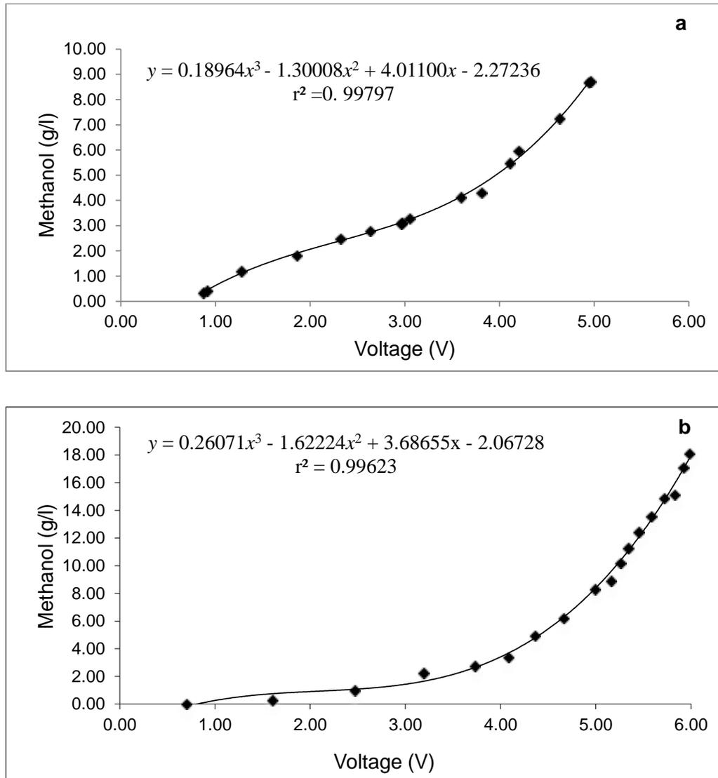
**Figure 3.** Correlation of voltage signal and methanol residue;  $y$  is methanol concentration (g/l),  $x$  is voltage signal (V) and  $r^2$  is correlation coefficient.
