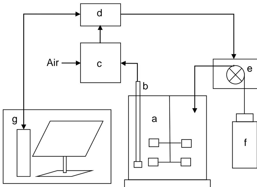
**Figure 1.** Schematic diagram of the developed methanol controlling system. **(a)** Bioreactor. **(b)** Methanol probe. **(c)** Methanol sensor unit. **(d)** Data acquisition (DAQ) device. **(e)** Peristaltic pump. **(f)** Methanol feed reservoir. **(g)** Computer set. Arrows indicate direction of signal and mass flow.
