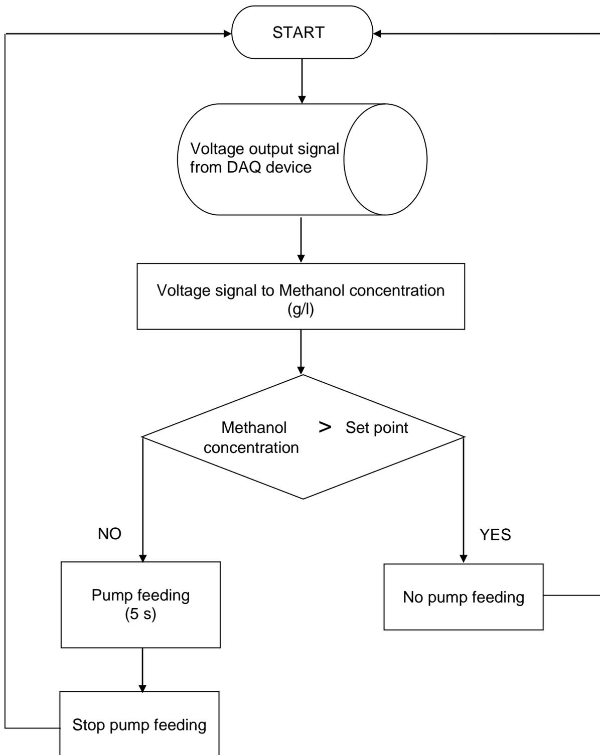
**Figure 2.** Schematic diagram of on-line methanol control system flow chart.
