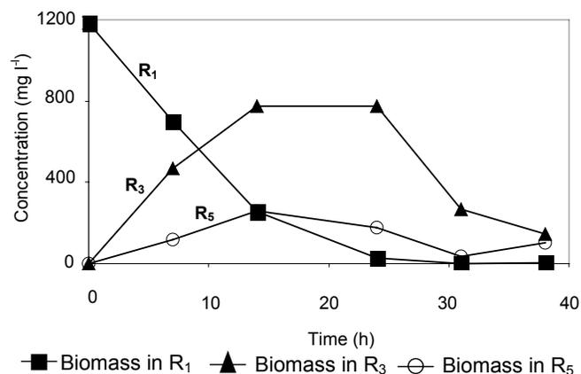
**Figure 2.** Kinetics of *A. niger* biomass migration through the reactors R<sub>1</sub>, R<sub>3</sub> and R<sub>5</sub>. Initial biomass concentration in the reactor R<sub>1</sub> was 1185 mg l<sup>-1</sup>.
