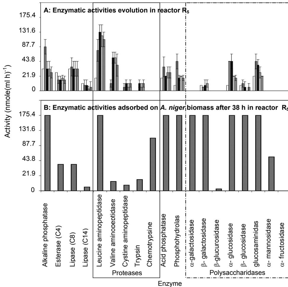
**Figure 3.** Enzymatics activities accumulated in reactor R<sub>5</sub> by *A. niger* under transitory conditions, when degrading a synthetic wastewater containing starch (250 mg l<sup>-1</sup>) and BSA (260 mg l<sup>-1</sup>). The initial biomass concentration in the reactor R<sub>1</sub> was 1185 mg l<sup>-1</sup>.
