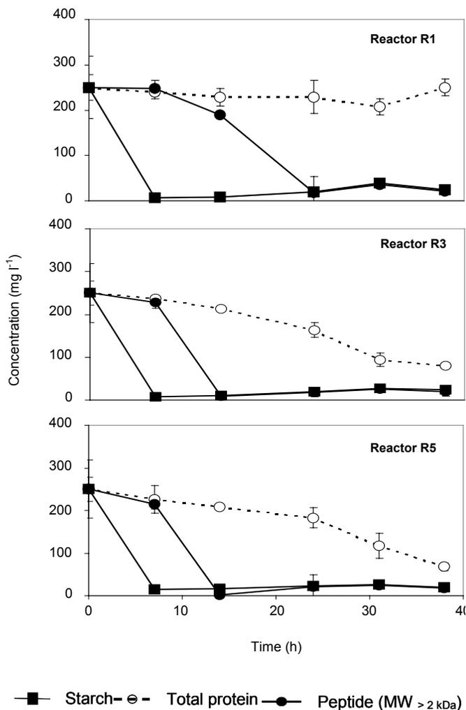
**Figure 1.** Kinetics of starch and BSA removal by *A. niger* under transitory conditions in reactors R<sub>1</sub>, R<sub>3</sub> and R<sub>5</sub>. Average initial synthetic wastewater composition: Starch, 250 mg l<sup>-1</sup>; BSA, 260 mg l<sup>-1</sup>. Initial biomass concentration in the reactor R<sub>1</sub> was 1185 mg l<sup>-1</sup>.
