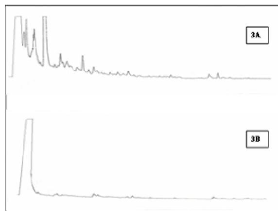
**Figure 3.** Gas chromatography analysis of hypochlorite stage before fungal treatment (A), and after fungal treatment under non-shaking conditions (B).
