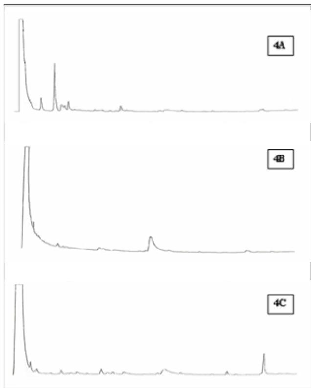
**Figure 4.** Gas chromatography analysis of composite bleachery effluent (CEH) before fungal treatment (A), after fungal treatment under non-shaking conditions (B) and under shaking conditions (C).
