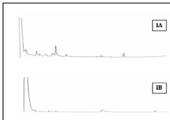
**Figure 1.** Gas chromatography analysis of chlorination stage before fungal treatment (A) and after fungal treatment under non-shaking conditions (B).
