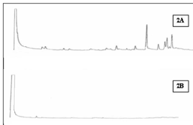
**Figure 2.** Gas chromatography analysis of extraction stage before fungal treatment (A) and after fungal treatment under non-shaking conditions (B).
