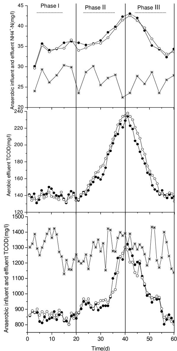
**Figure 2.** Experimental performances of system A and B. Aerobic excess sludge recirculation ratio for system A: Phase I (1 - 20 d): 60%; Phase II (21 - 40 d): 70%; Phase III (41 - 60 d): 60%. Ratio of system B: Phase I: 40%; Phase II: 50%; Phase III: 40%. Note: "—\*"— Influent, —●— System A (SRT: 10 d), —○— System B (SRT: 25 d)"
