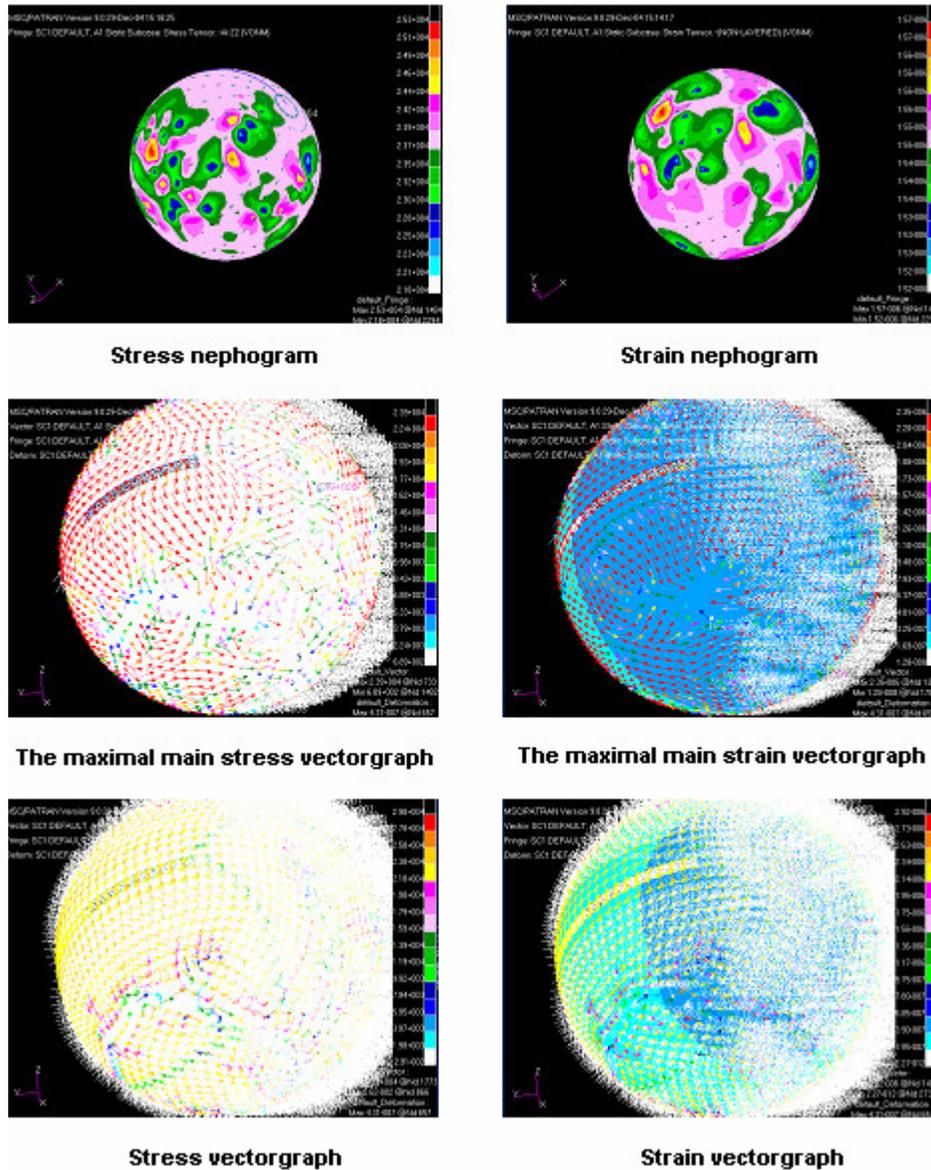
**Figure 2.** Stress and strain graphs of cranial cavity by ignoring the viscoelasticity of human skull and dura mater with finite-element software MSC\_ PATRAN/NASTRAN when ICP variation is raised up to 2.5 kPa.
