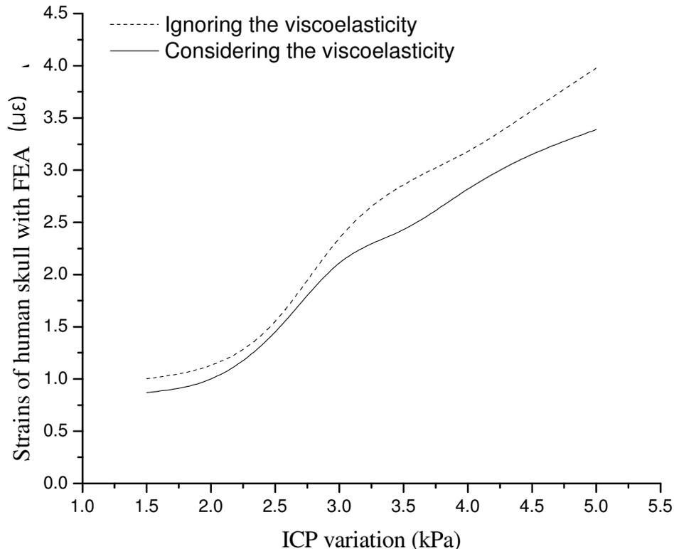
**Figure 5.** The strains of cranial cavity by respectively ignoring and considering the viscoelasticity of human skull and dura mater with the finite-element software MSC\_PATRAN/NASTRAN and ANSYS with the changing ICP from 1.5 to 5 kPa.
