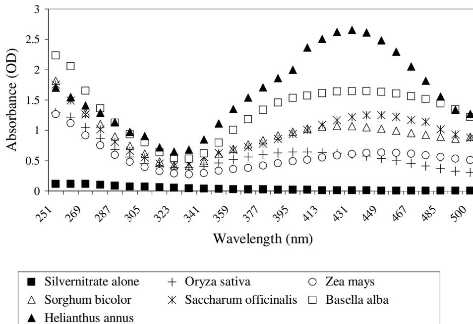
**Figure 1.** UV visible absorption spectra recorded as a function of time of reaction at  $10^{-3}$  M aqueous solution of silver nitrate with different leaf extracts. The silver nanoparticle formation was monitored through UV-Visible absorption spectroscopy (excitation band near 430 nm for silver) at regular intervals as a function of time of reaction on a Genesys 10-UV Thermo Spectrophotometer operated at a resolution of 3 nm.
