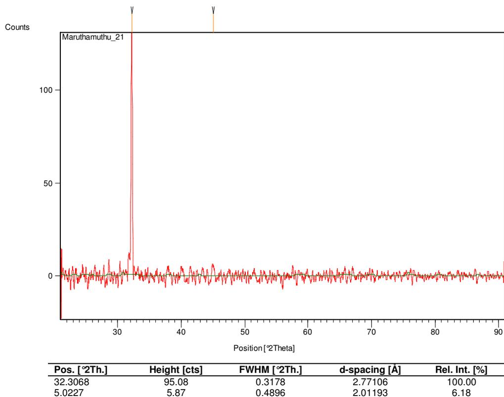
**Figure 2.** The XRD Image of silver nanoparticles synthesised using Sunflower leaf extract. The diffraction patterns were obtained by measurement of angles at which X-ray beam is diffracted by the crystalline phases in the specimen. X-ray diffraction (XRD) measurement of the bio-reduced silver nitrate solution drop-coated on glass substrate bio-film was carried out on a Philips PW 1830 instrument operating at 40 kV and a current of 30 mA with Cu  $K_{\alpha}$  radiation.
