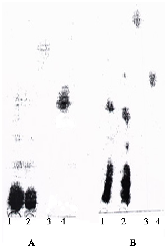
Figure 10. Paper chromatography of hydrolysis products of alpha amylase of strains SCH and 267CH. A: Chromatogram developed for hydrolysis products obtained after 40 minutes reaction time. B: Chromatogram developed for hydrolysis products obtained after 140 minutes reaction time. 1: Hydrolysis products by alpha amylase of strain SCH. 2: Hydrolysis products by alpha amylase of strain 267CH. 3: Glucose. 4: maltose.
