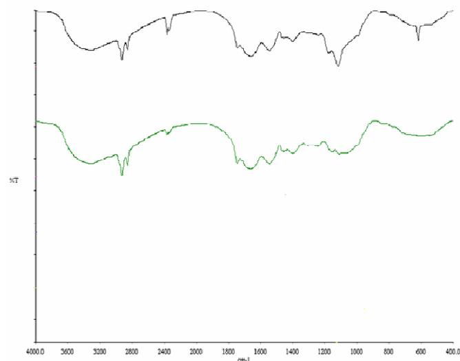
**Figure 5.** IR Spectra of pullulan produced by *Aureobasidium pullulans* from matured coconut water (top) and coconut milk (bottom).
