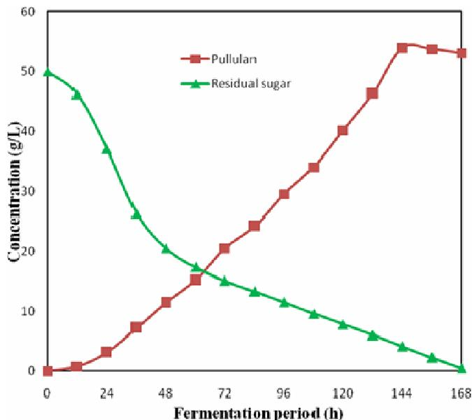
**Figure 3.** Effect of fermentation period during pullulan production from coconut milk in batch study using *Aureobasidium pullulans*.
