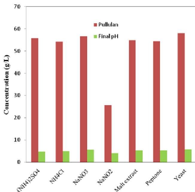
**Figure 4.** Effect of nitrogen (synthetic) source on pullulan production using *Aureobasidium pullulans*.
