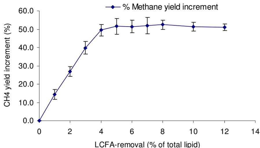
**Figure 3.** The trend in percentage methane increment with percentage LCFA removal
