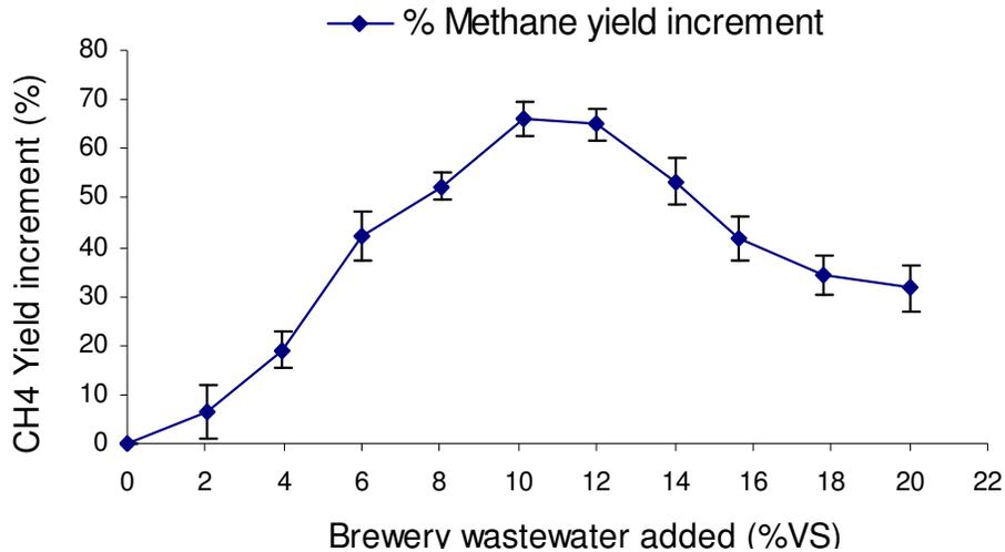
**Figure 2.** Extent of methane yield increment with addition of various amounts (VS) of brewery wastewater.
