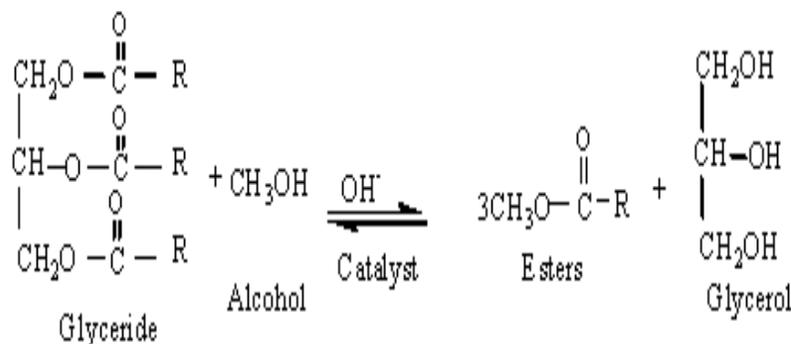
Figure 1. Transesterification reaction.
