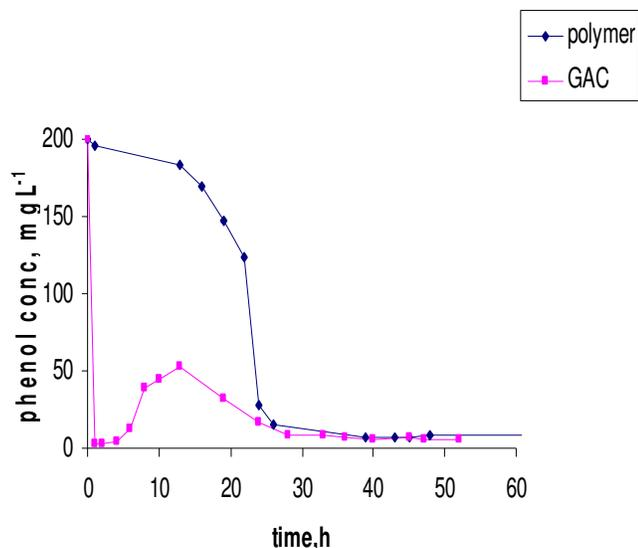
**Figure 3.** Effluent phenol concentration during startup period (Influent phenol conc. = 200 mg/L; dilution rate = 0.733 h<sup>-1</sup>).
