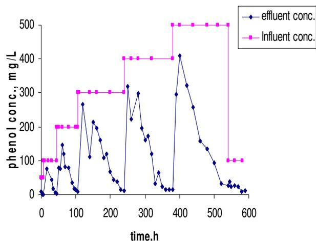
**Figure 5.** Influent phenol concentration and steady state effluent concentration with time for dilution rate of 1.465 h<sup>-1</sup>.
