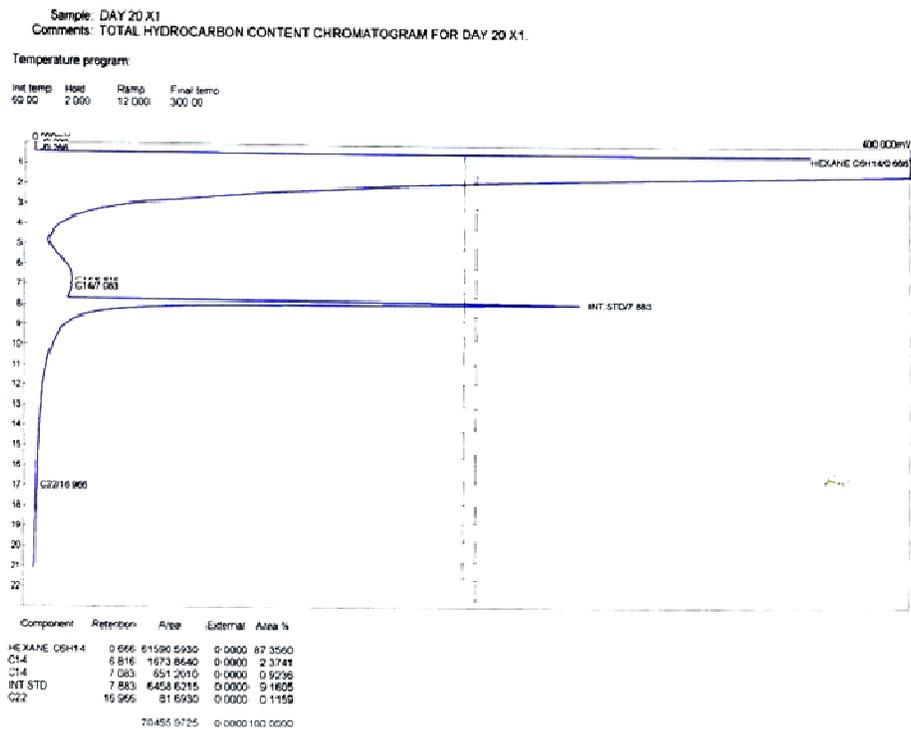
Figure 17. GC profile of detergent residues (microcosm experiment). X1 = Fungal consortium.
