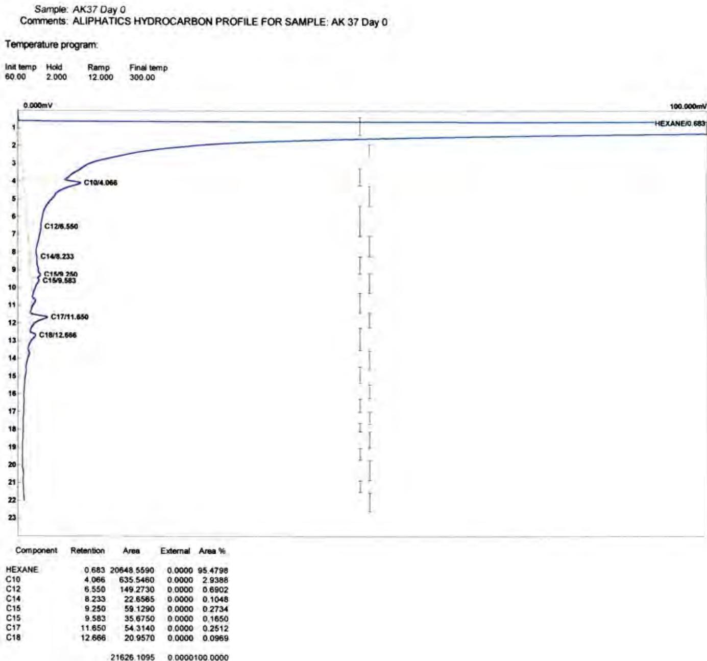
Figure 14. GC profile of detergent residues (shake flask experiment). AK 37 = ELEPHANT detergent.
