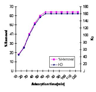
**Figure 2.** Effect of contact time on adsorption of Cr metal at 300 K (500 ppm, dosage 0.5 g/50 ml) using activated pure rice hulls.
