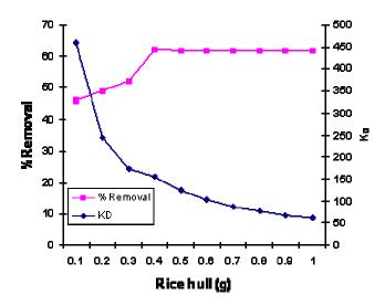
Figure 1. Effect of activated pure rice hulls concentration (amount) on adsorption of Cr metal at 300K (500 ppm, contact time 60 min).
