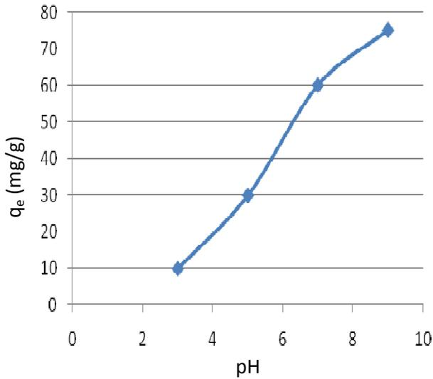
**Figure 2.** Effect of pH on the sorption of basic dye at 30°C using bamboo as adsorbent.
