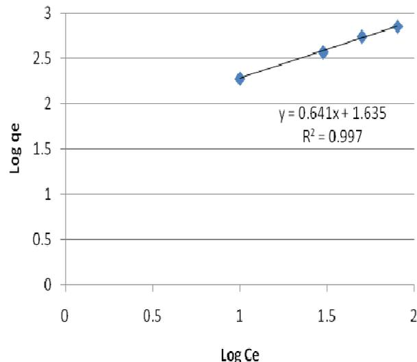
**Figure 6.** Freundlich isotherm for the sorption of basic dye 30°C using bamboo as adsorbent.
