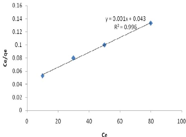
**Figure 5.** Langmuir isotherm for the sorption of basic dye at 30°C using bamboo as adsorbent.
