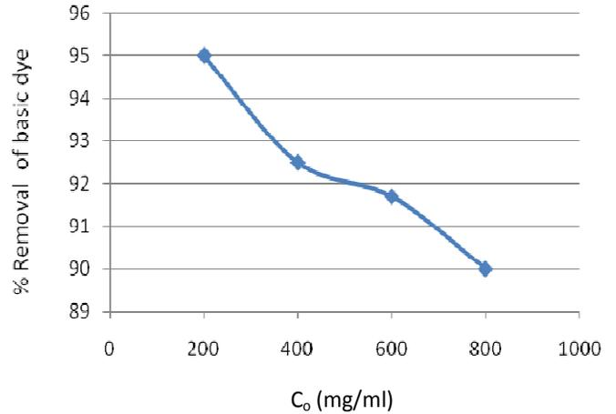
**Figure 4.** Effect of initial dye concentration on its removal using bamboo as adsorbent.
