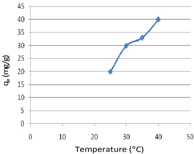
**Figure 3.** Effect of temperature on the sorption of basic dye at 30°C using bamboo as adsorbent.
