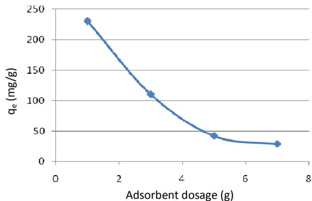
**Figure 1.** Effect adsorbent (bamboo) dosage on the sorption of basic dye at 30°C.
