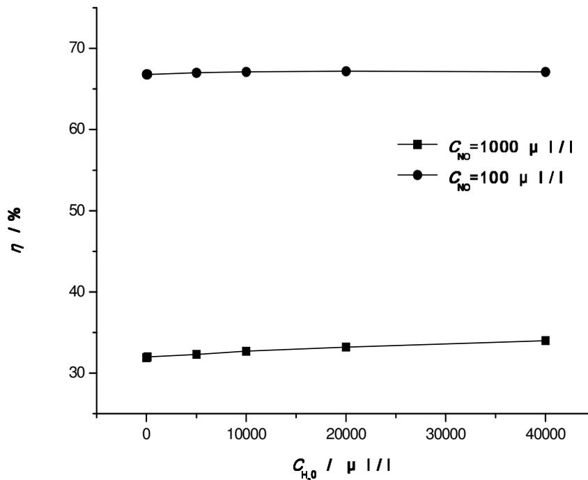
Figure 4. Effect of moisture content on NO reduction.
