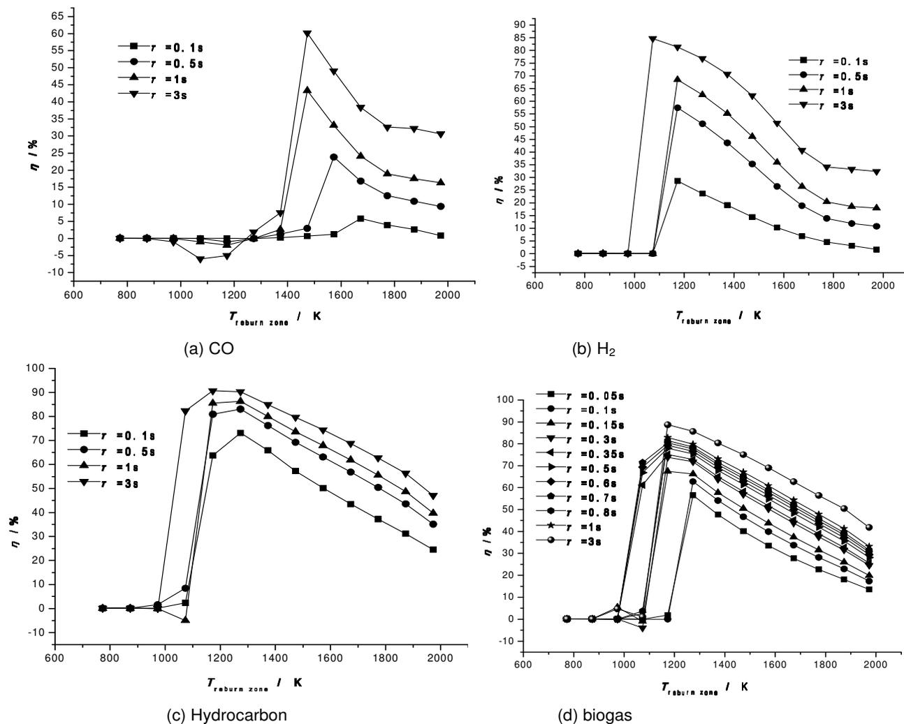
Figure 2. Effect of temperature on NO reduction for different reburning fuels.
