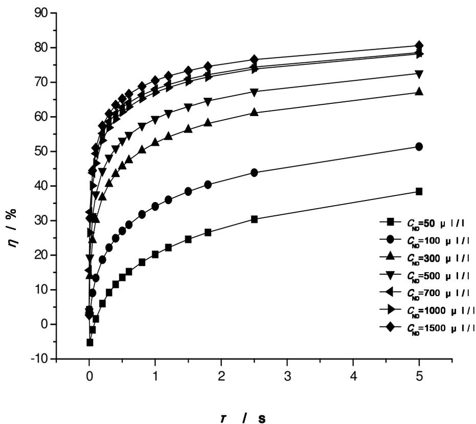
**Figure 3.** Effect of residence time and initial NO concentration on NO reduction.
