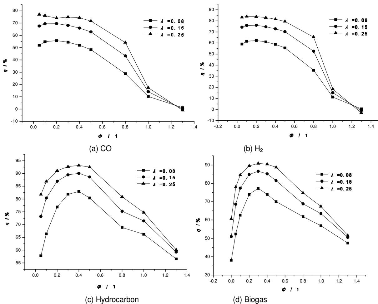
**Figure 1.** Effect of oxygen content and reburn fuel ratio on NO reduction for different reburning fuels.
