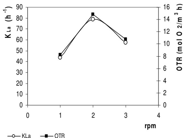
**Figure 1.** Volumetric mass transfer coefficient for O<sub>2</sub>, h<sup>-1</sup>, and OTR, mol m<sup>-3</sup> h<sup>-1</sup>, at different agitation rates (1, 2 and 3 on the x-axis represents 126, 226 and 300 rpm, respectively).
