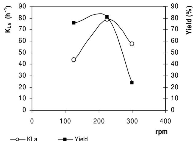
**Figure 3.** Volumetric mass transfer coefficient for O<sub>2</sub>, h<sup>-1</sup>, and yield, at different agitation rates.
