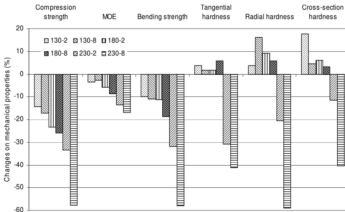
**Figure 3.** Changes on mechanical properties as a function of treatment temperature (130, 180 and 230°C) and time (2 and 8 h).
