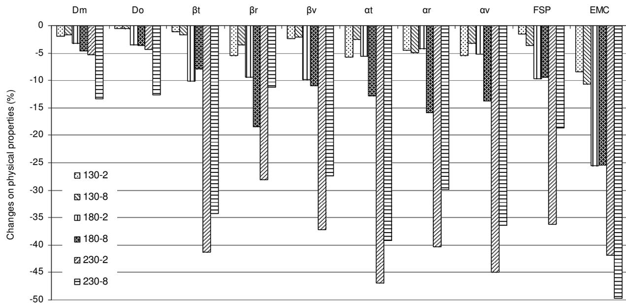
**Figure 2.** Changes (%) in physical properties as a function of treatment temperature (130, 180 and 230°C) and time (2 and 8 h).
