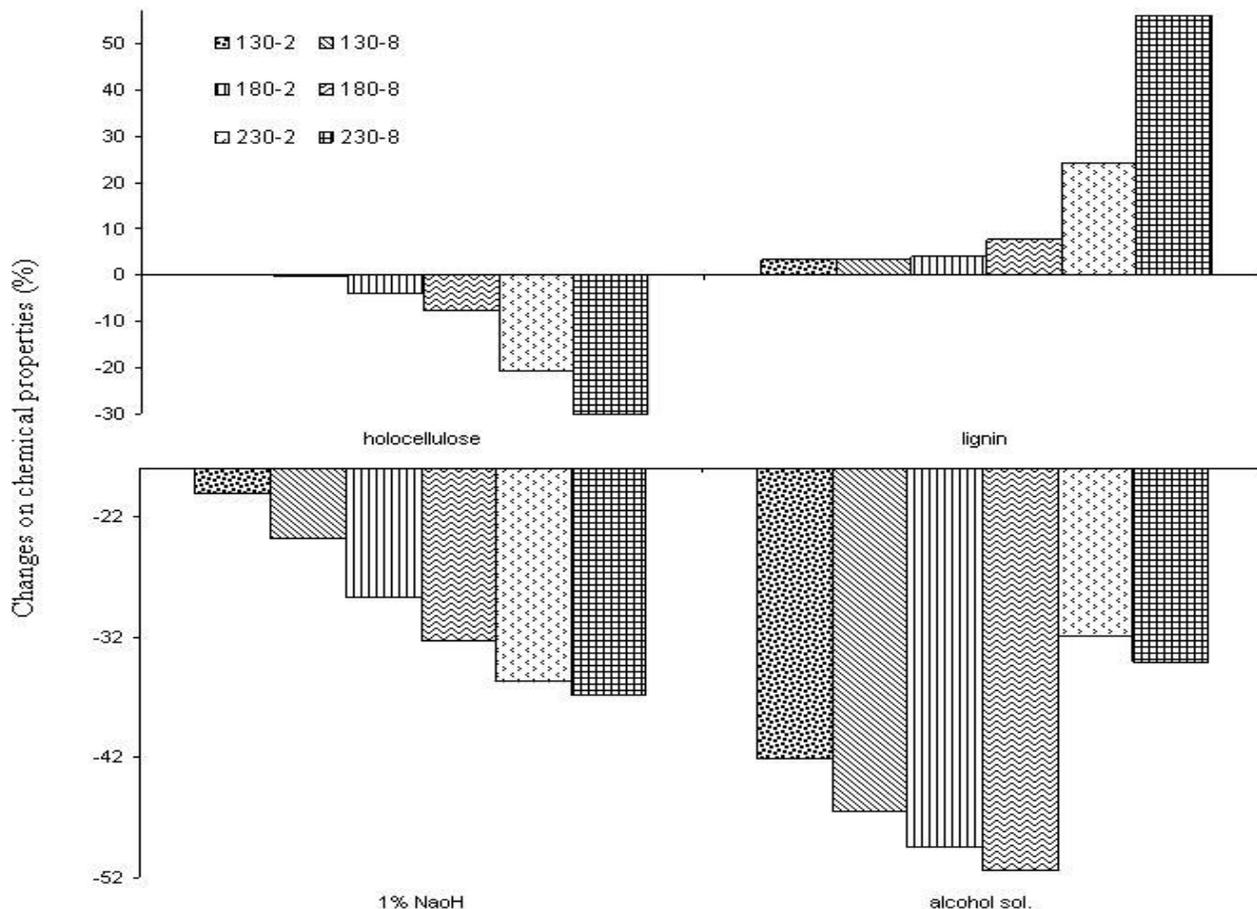
**Figure 4.** Changes on chemical properties as a function of heat treatment (130, 180 and 230°C) and time (2 and 8 h).
