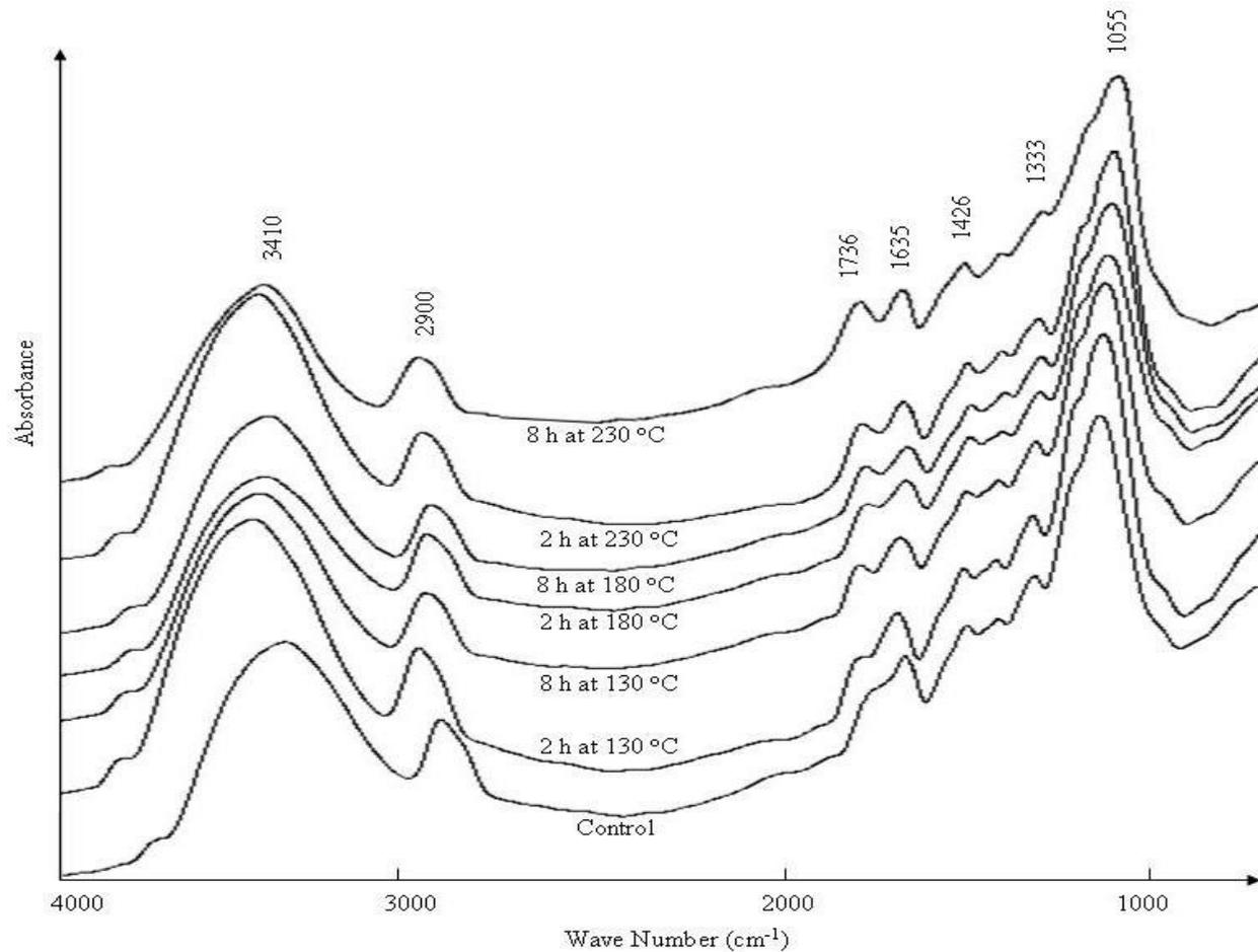
**Figure 5.** FT-IR spectra of untreated and heat treated Anatolian black pine wood.
