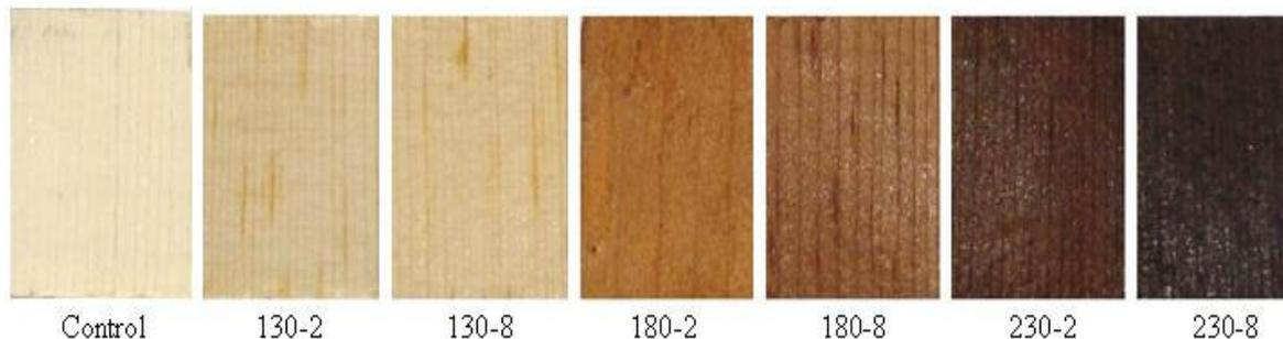
**Figure 1.** Color change with increasing heat treatment temperature (130, 180 and 230°C) and time (2 and 8 h).
