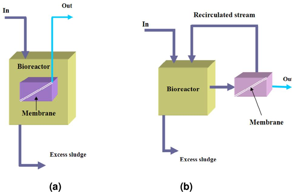
Figure 3. Submerged MBR (a) and sidestream MBR (b).
