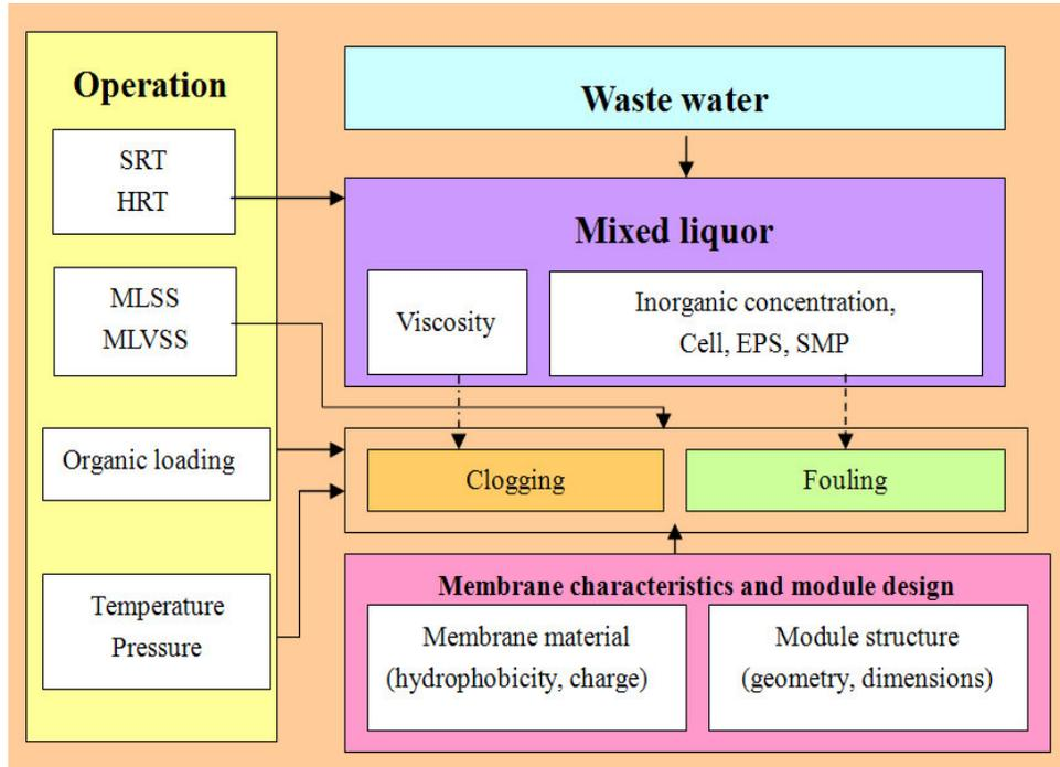
Figure 2. Inter-relationships between MBR parameters and fouling.
