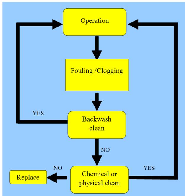
**Figure 1.** Membrane cleaning protocols. After a long time operation of MBR, fouling or/and clogging occur. Usually, backwash clean is used to mitigate fouling. Chemical or physical clean will be needed if backwash does not work. After several times of chemical or physical clean, the membrane should be replaced if its performance were not recovered.
