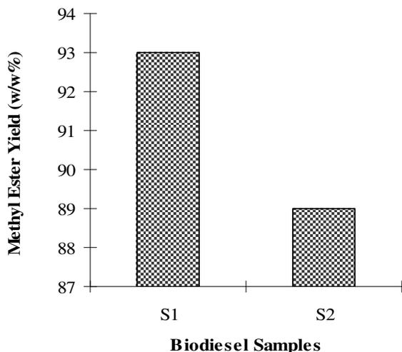
**Figure 1.** Comparison of methyl ester yield obtained from oil sample for which methoxide was treated with molecular sieve before transesterification with that not treated with molecular sieve. S1: Biodiesel obtained from kernel oil transesterification when methoxide was treated with molecular sieve. S2: Biodiesel obtained from kernel oil transesterification when methoxide was not treated with molecular sieve.
