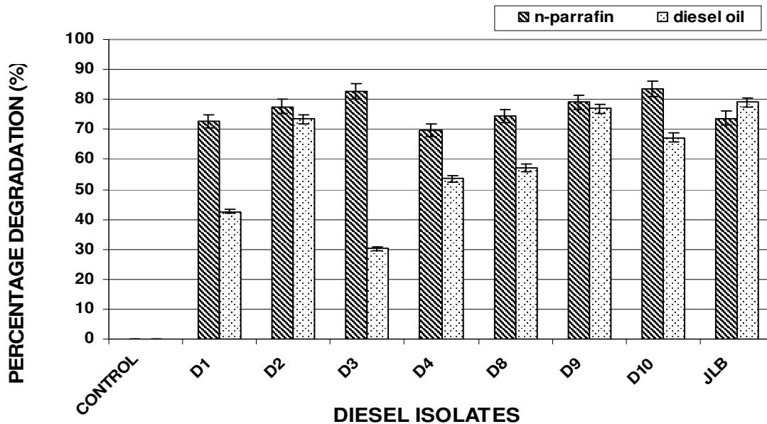
**Figure 1.** The percentage of n-paraffin and diesel degradation by the bacterial isolates after a 20-day incubation at 30 °C, 160 rpm<sup>-1</sup>.
