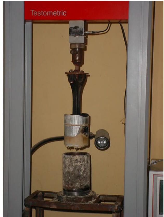
**Plate 1.** The Piston-Cylinder assembly on the Universal Testing Machine.
