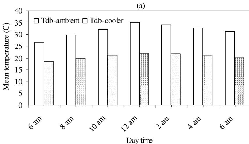
**Figure 2. (a).** The effect of daytime on the average environmental and evaporative cooler temperatures (°C) during storage of carrots.
