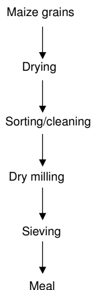
Figure 2. Flow diagram for the production of maize meal (Okoruwa, 1995).
