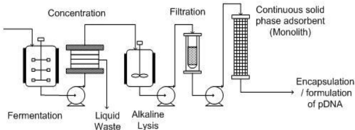
**Figure 2.** Proposed process flow sheet for single-stage purification of plasmid-based therapeutic products (Danquah et al., 2008b).
