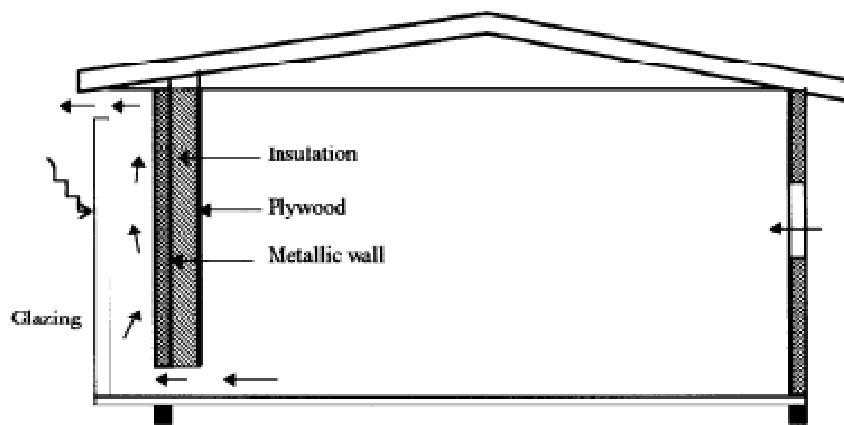
**Figure 4.** Schematic representations of the passive solar house and natural ventilation by metallic solar wall
