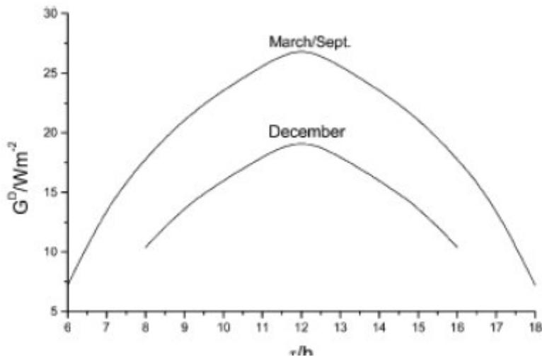
**Figure 8.** Ground irradiance from diffuse (sky) radiation from a clear sky at the shortest winter day and at equinox.
