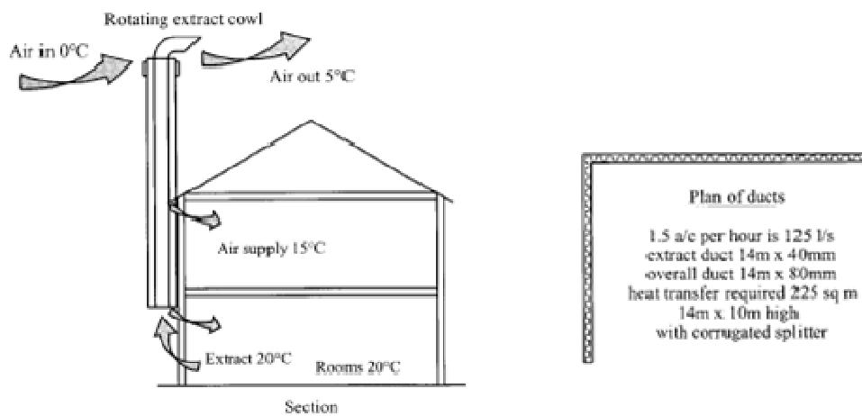
**Figure 3.** Ventilation duct supply and extract wraps around the building.
