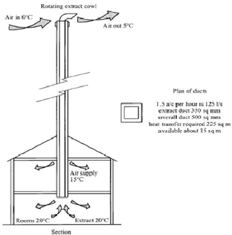
**Figure 2.** Small house natural ventilation with heat reclaim (A very tall chimney).
