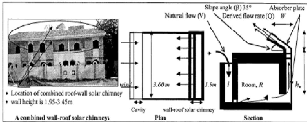
**Figure 6.** A combined wall-roof solar chimney incorporated into a residential building night ventilation.
