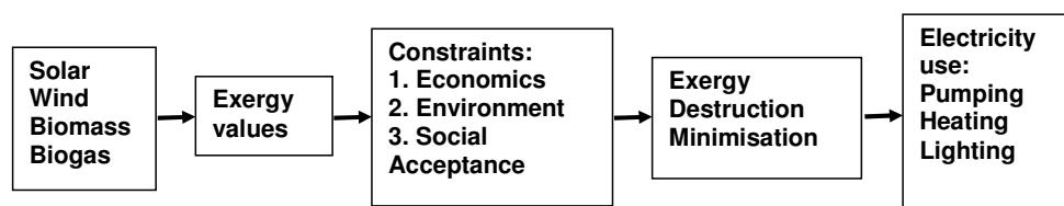
**Figure 10.** Exergy based optimal energy model.
