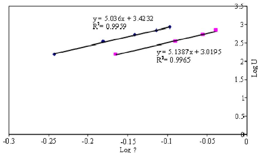
**Figure 8.** Linear regression plot of Richardson-Zaki correlation. Linear regression plot of the Richardson-Zaki correlation as described by Equation 8 were demonstrated on the acetate binding buffer pH 5 (♦) and 4.5 % (w/v) wet biomass unclarified feedstock (■). Richardson-Zaki coefficient ( $n$ ) obtained from the slope of logarithm of superficial velocity ( $\log U$ ) versus logarithm of bed voidage ( $\log \epsilon$ ).
