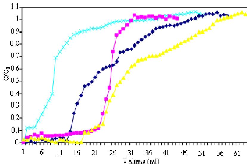
**Figure 9.** Effect of flow rate to dynamic capacity lipase in EBA
