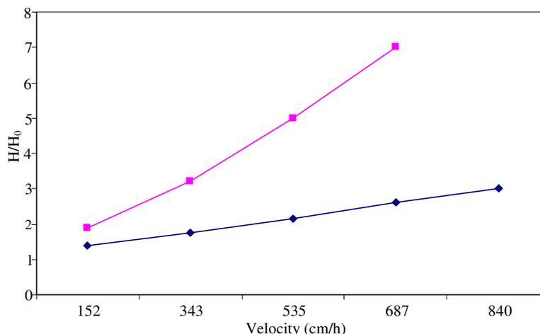
**Figure 7.** Bed expansion characteristic. Bed expansion characteristic of STREAMLINE Direct HST adsorbent by acetate binding buffer pH 5 (♦) and 4.5% (w/v) wet biomass unclarified feedstock (■). H denoted expanded bed height and  $H_0$  denoted settled bed height.
