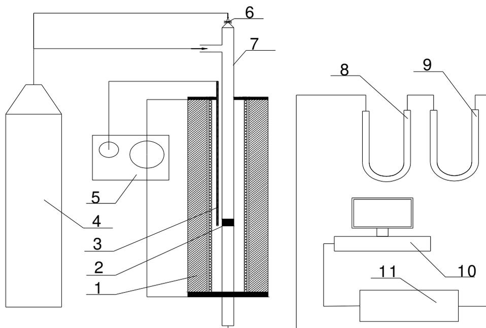
**Figure 1.** Schematic diagram of the experimental system. 1 = Tube furnace; 2 = Orifice; 3 = Thermacouple; 4 = Nitrogen; 5 = Temperature controller; 6 = Feeder of biomass and metal-addition; 7 = Quartz reactor; 8 = Filter-1; 9 = Filter-2; 10 = Data acquisition computer; 11 = FTIR analyzer.
