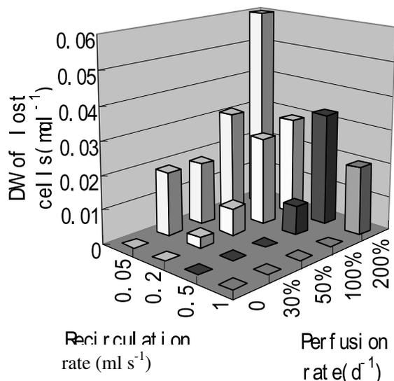
**Figure 2.** Effect of perfusion rate and cell suspension recirculation speed on cell retention efficiency in bioreactor. The cell retention efficiency is defined as:  $(C_M - C_L)/C_M$ , where  $C_M$  is cell density in bioreactor, and  $C_L$  is cell density in discarded medium.
