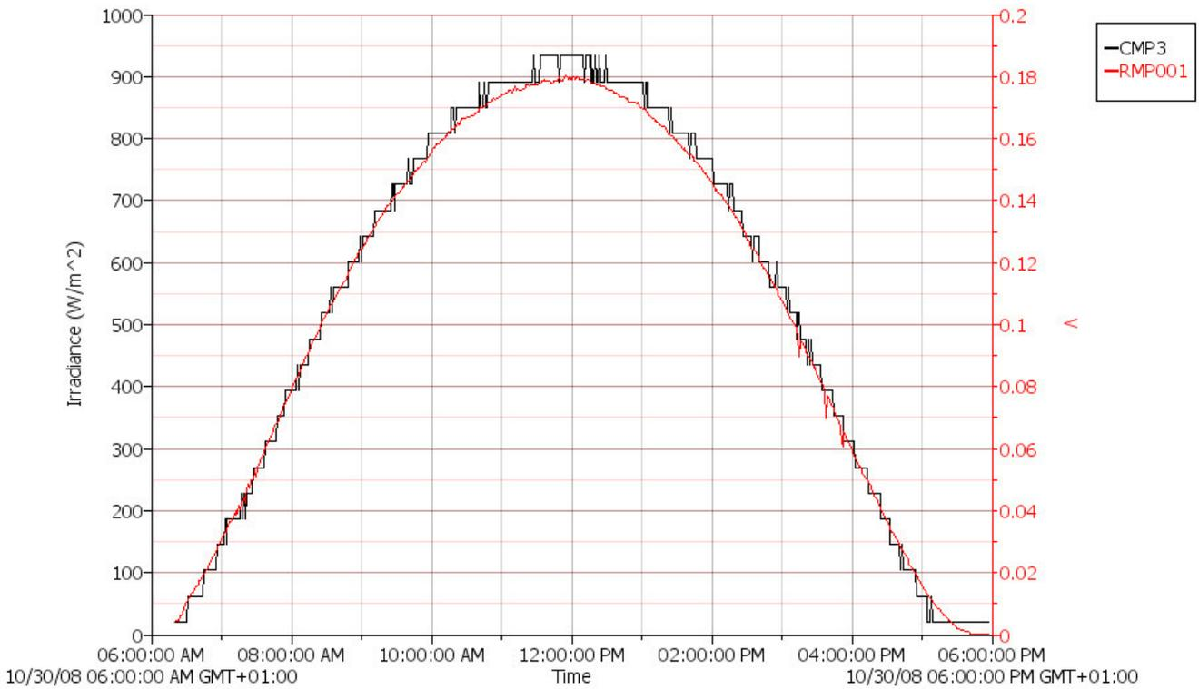
Figure 5. Graph of Solar Radiation measured with CMP3 and RMP001 versus Time on 30<sup>th</sup> October, 2008.
