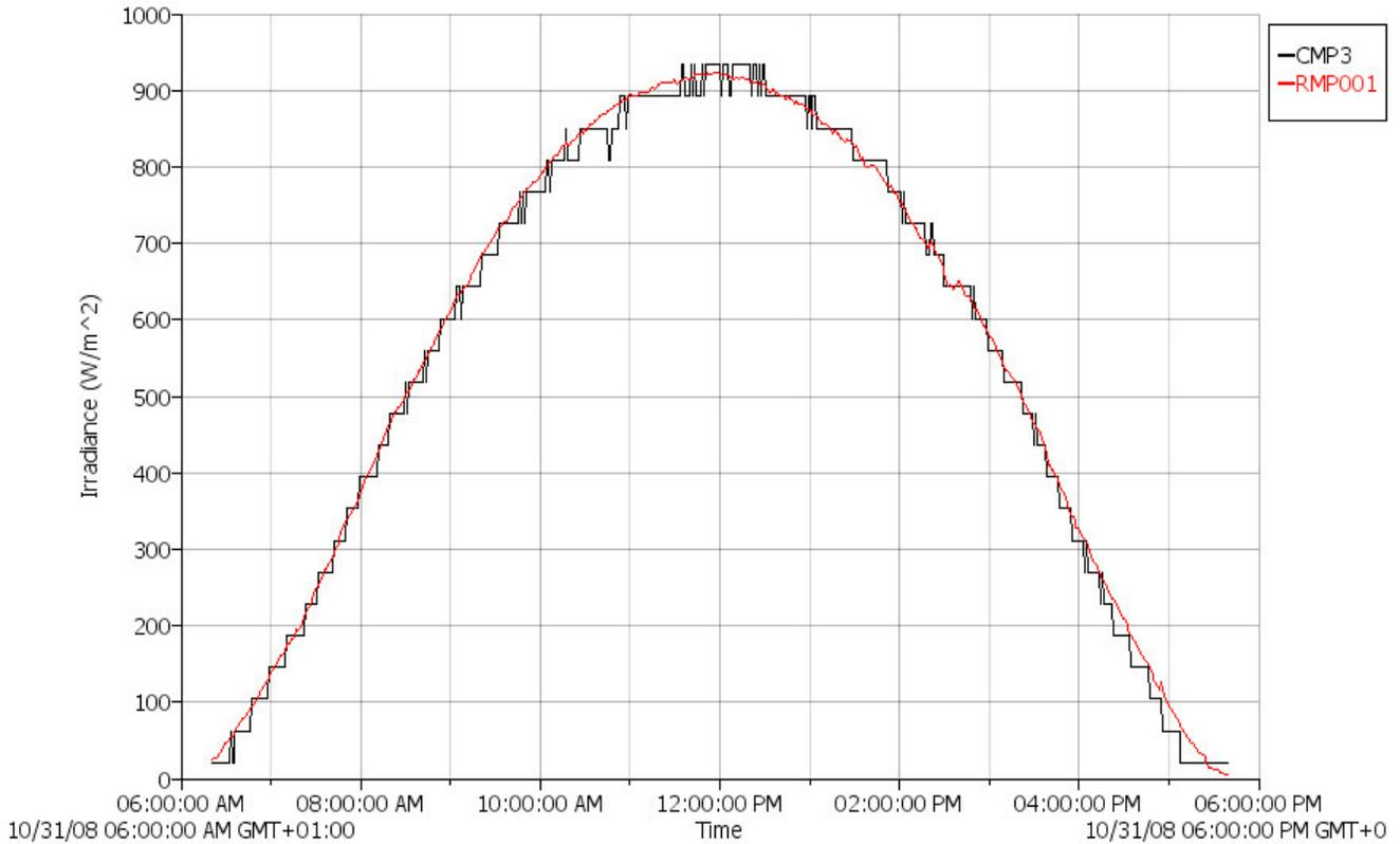
**Figure 6.** Insolation graph covering 31<sup>st</sup> October, 2008 at Adamawa State University, Mubi using both CMP3 and RMP001 after calibration adjustments and model maximum values of insolation have been entered.
