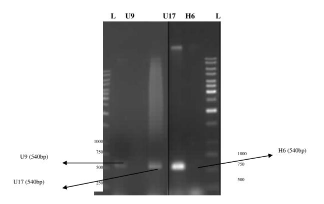
Figure 2. Amplification of phaC gene fragment from U9, U17 and H6 bacterial isolates.
