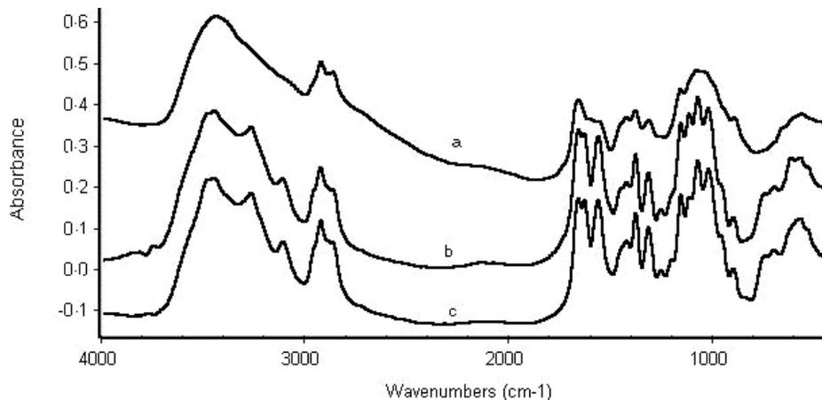
**Figure 2.** FT-IR Spectra of a: Chitosan, b: Chitosan-Cd complex and c: Chitosan-Pb complex.
