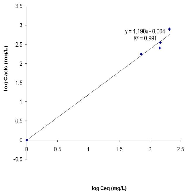
**Figure 6.** Freundlich plot of adsorption of Pb<sup>2+</sup> onto chitosan.
