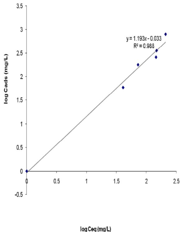
**Figure 7.** Freundlich plot of adsorption of Cd<sup>2+</sup> onto chitosan.
