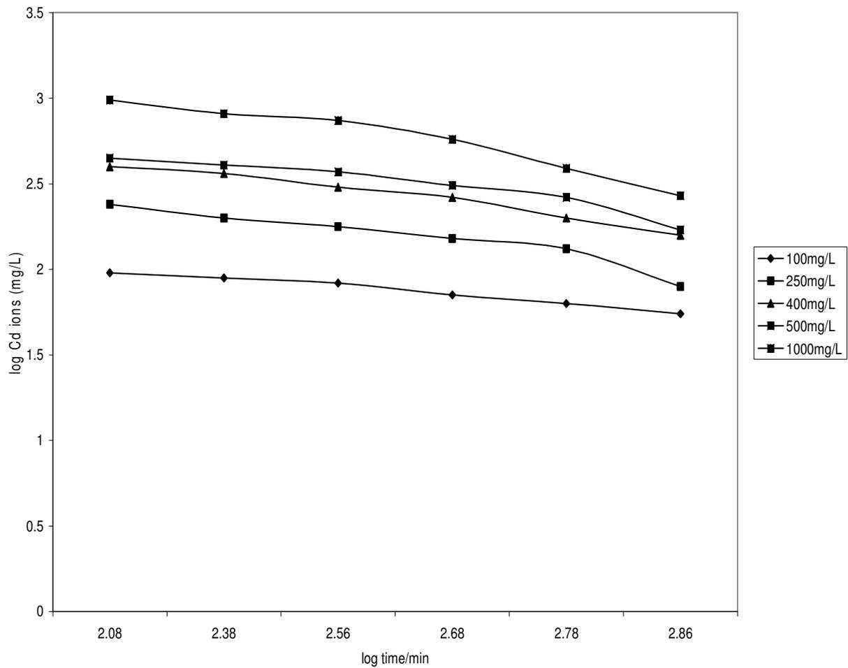
**Figure 5.** Adsorption kinetics of cadmium ions on chitosan at different initial concentrations  $[Cd^{2+}] = 100, 250, 400, 500, 1000$  (mg/l), pH 4.5, stirring speed= 180 rpm.
