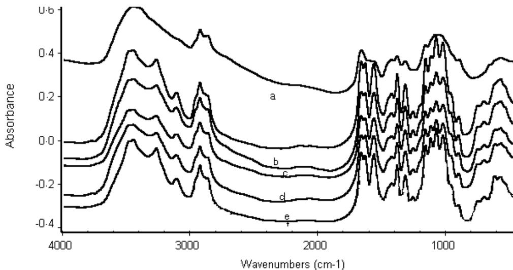
**Figure 3.** FT-IR Spectra of Chitosan-mixed metal complexes Cd and Pd in solutions of equimolar concentrations (a: 0, b: 100, c: 250, d: 400, e: 500 and f: 1000 mg/L).
