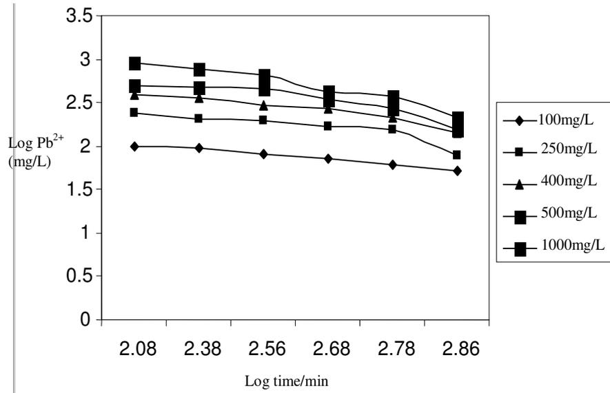
**Figure 4.** Adsorption kinetics of lead ions on chitosan at different initial concentrations  $[Pb^{2+}] = 100, 250, 400, 500, 1000$  (mg/l), pH 4.5, stirring speed = 180 rpm.
