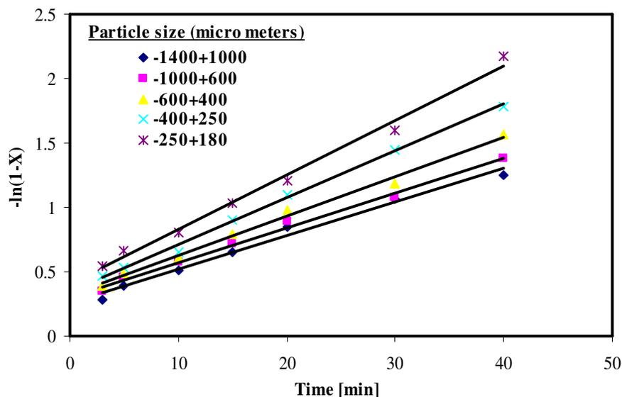
**Figure 9.** Agreement of experimental data with the first-order pseudo homogeneous kinetic model [- ln (1 - X)] versus time for particle size.
