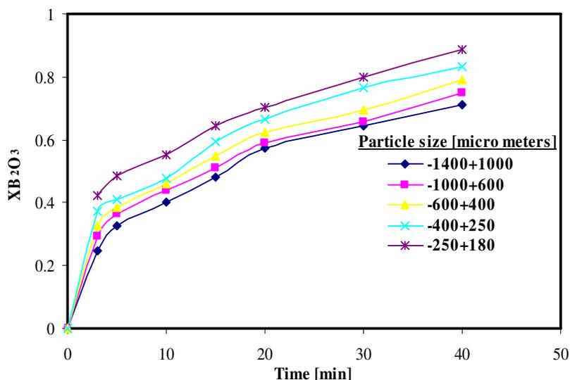
**Figure 1.** Effect of the particle size on dissolution rate (temperature: 303 K; acid concentration: 2 M; solid/liquid ratio: 0.5/50 g/ml; stirring speed: 400 rpm).
