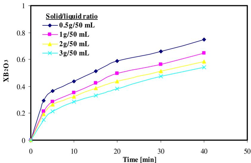
**Figure 5.** Effect of the solid/liquid ratio on dissolution rate (temperature: 303 K; particle size: -1000+600 μm; acid concentration 2 M; stirring speed: 400 rpm).
