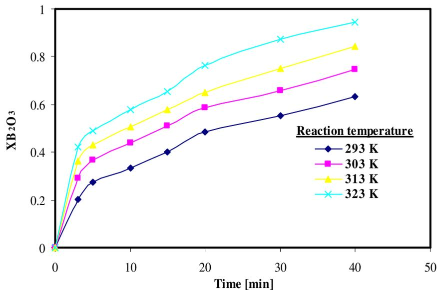
**Figure 7.** Effect of the reaction temperature on dissolution rate (particle size: - 100 + 600 μm; solution concentration 2 M; solid/liquid ratio 0.5 g/ml; stirring speed: 400 rpm).
