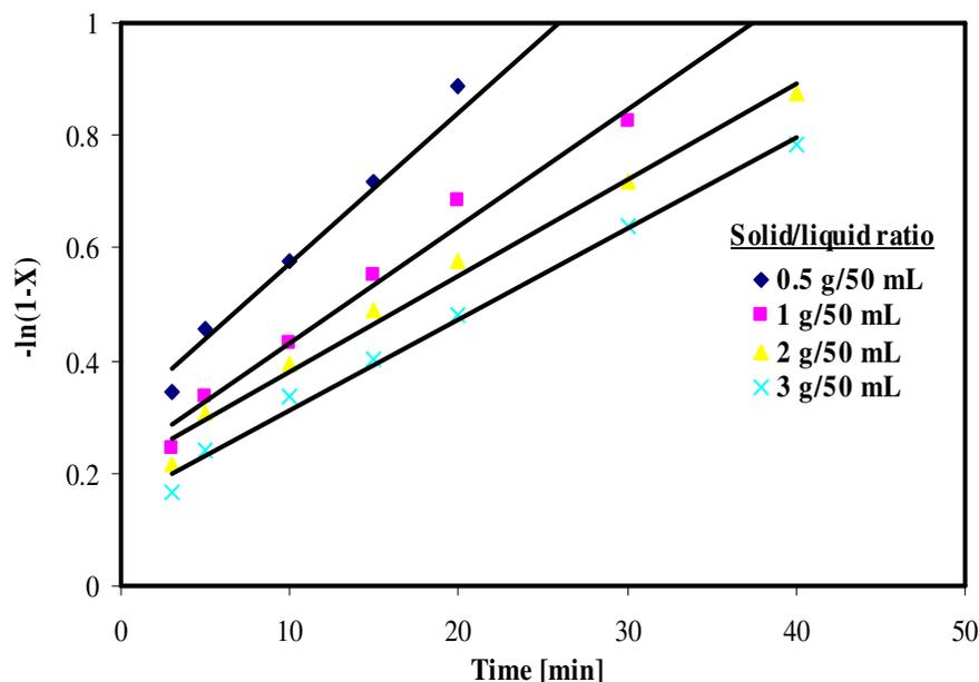
**Figure 11.** Agreement of experimental data with the first-order pseudo homogeneous kinetic model  $[-\ln(1-X)]$  versus time for solid/liquid ratio.
