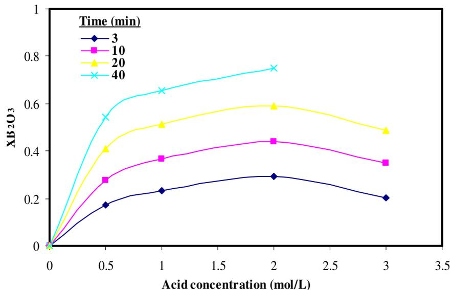
**Figure 4.** Effect of the acid concentration on conversion fraction at certain times (temperature: 303 K; particle size: - 1000 + 600 μm; solid/liquid ratio: 0.5/50 g/ml; stirring speed: 400 rpm).
