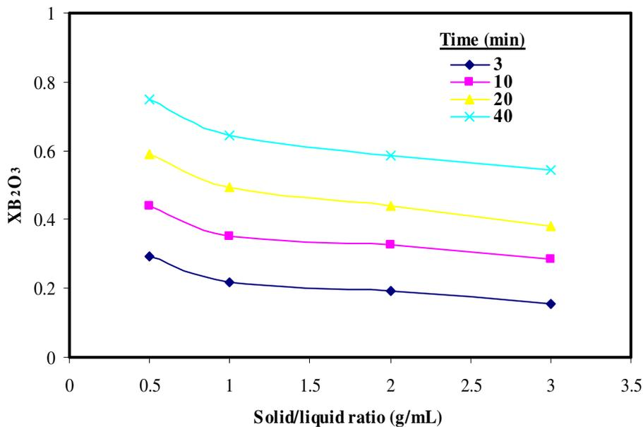
**Figure 6.** Effect of the solid/liquid ratio on conversion fraction at certain times (temperature: 303 K; particle size: -1000 + 600 μm; acid concentration 2 M; stirring speed: 400 rpm).
