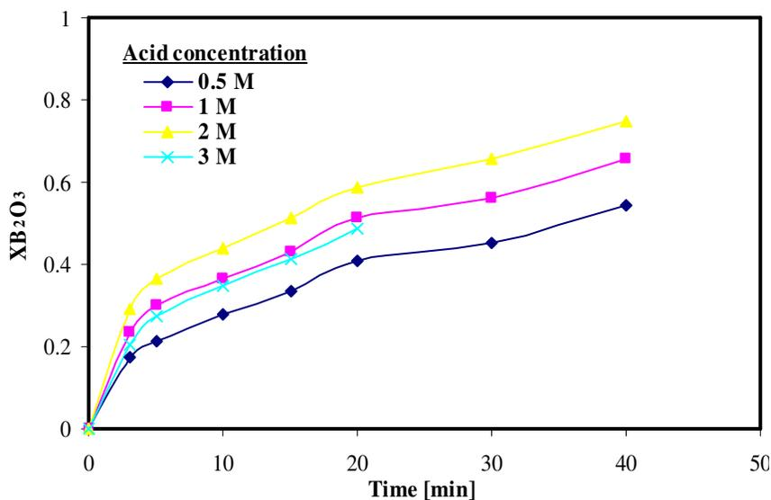
**Figure 3.** Effect of the acid concentration on conversion fraction (temperature: 303 K; particle size: -1000+600  $\mu\text{m}$ ; solid/liquid ratio: 0.5/50 g/ml; stirring speed: 400 rpm).
