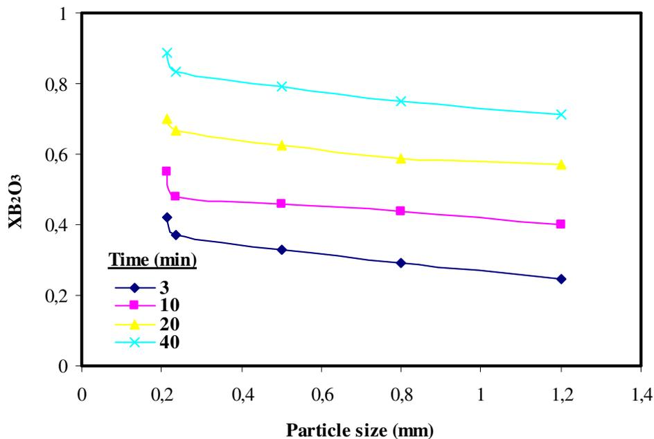
**Figure 2.** Effect of the average particle size on dissolution rate at certain times (temperature: 303 K; acid concentration: 2 M; solid/liquid ratio: 0.5/50 g/ml; stirring speed: 400 rpm).
