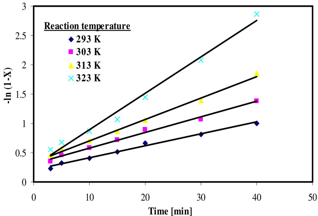
**Figure 12.** Agreement of experimental data with the first-order pseudo homogeneous kinetic model  $[-\ln(1 - X)]$  versus time for reaction temperature.
