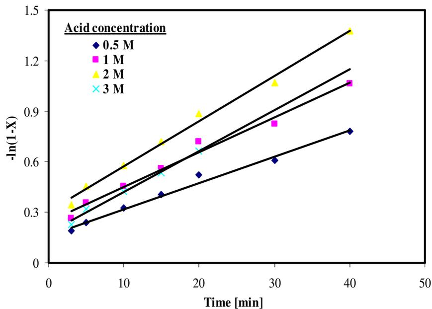
**Figure 10.** Agreement of experimental data with the first-order pseudo homogeneous kinetic model  $[-\ln(1-X)]$  versus time for acid concentration.
