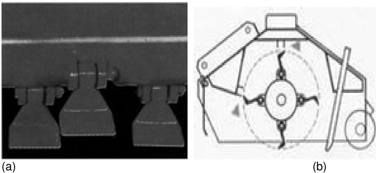
**Figure 2.** Hammer-type blades of the splined-type stalk chopper.
