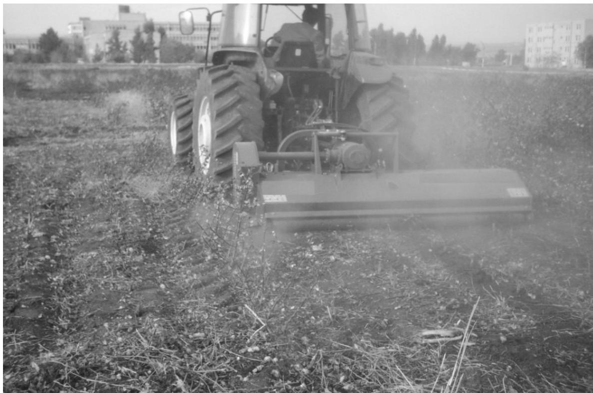
**Figure 1.** Splined-type stalk chopper.
