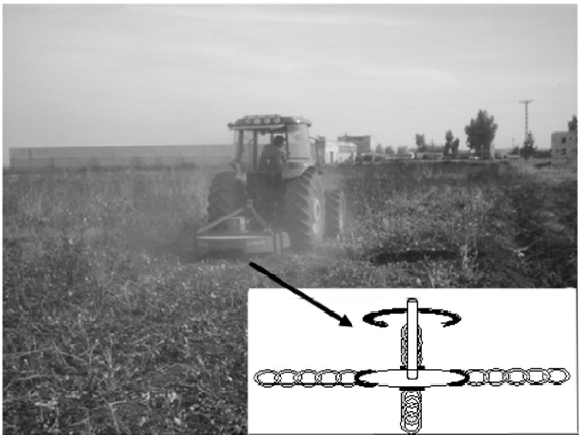
**Figure 3.** Chained-type stalk chopper.
