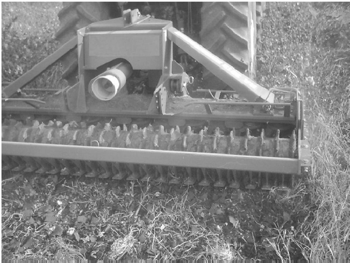
**Figure 4.** Vertical-blade rotating dredge.
