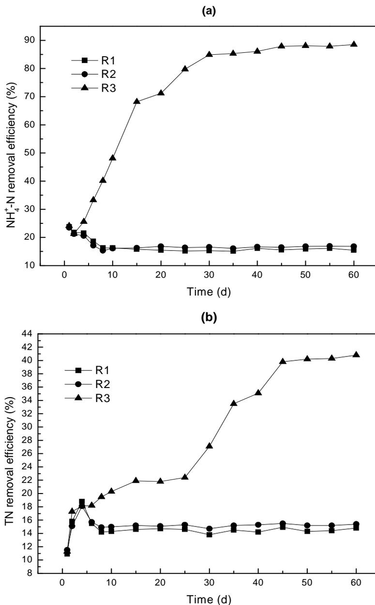
**Figure 6.** Nitrification-denitrification of the reactors in a 60-day operation: (a) NH<sub>4</sub><sup>+</sup>-N removal efficiency; (b) TN removal efficiency; R1: acetate-fed, maintained in acid pH; R2: glucose-fed, maintained in acid pH; R3: glucose-fed, maintained in alkaline pH.
