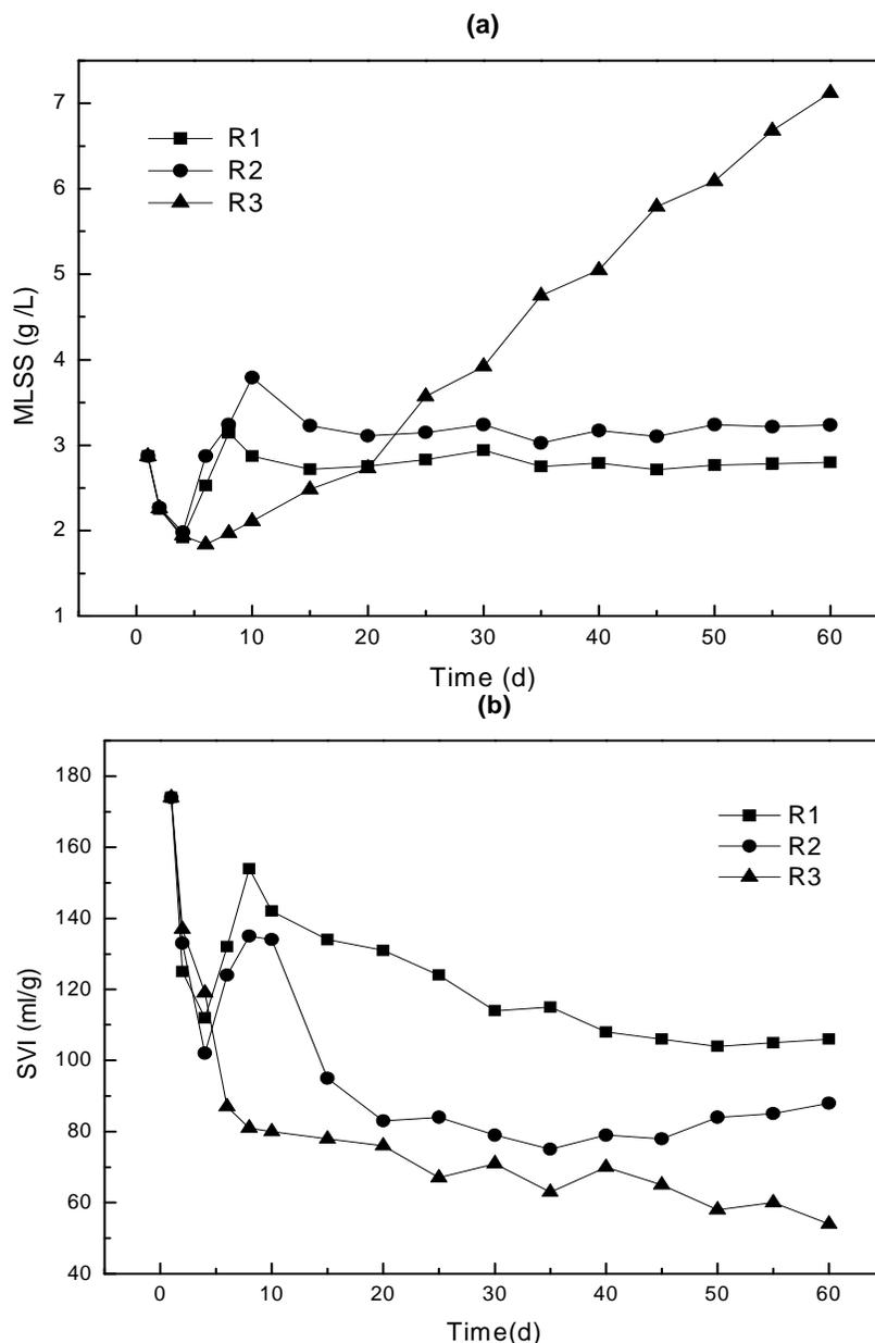
**Figure 5.** MLSS and SVI of aerobic granules: (a) mixed liquor suspended sludge (MLSS); (b) sludge volume index (SVI); R1: acetate-fed, maintained in acid pH; R2: glucose-fed, maintained in acid pH; R3: glucose-fed, maintained in alkaline pH.
