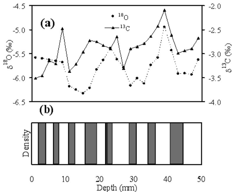
**Figure 5.** Skeletal (a)  $\delta^{18}\text{O}$  and  $\delta^{13}\text{C}$  values of coral skeleton and (b) growth increment and density band of the coral sample where ash, white and black line indicate high density band, low density band and ARS line, respectively.
