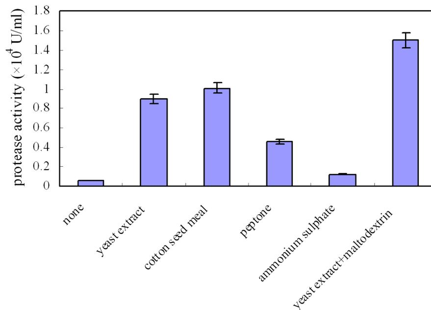
**Figure 2.** Effect of different nitrogen sources on alkaline protease production by *B. alcalophilus* TCCC11004. Cultivations were performed for 50 h at 34°C in initial medium containing (g/l): maltodextrin 55, nitrogen source 17.5,  $K_2HPO_4$  18, trisodium citrate 3.3, and  $CaCl_2$  2.6.
