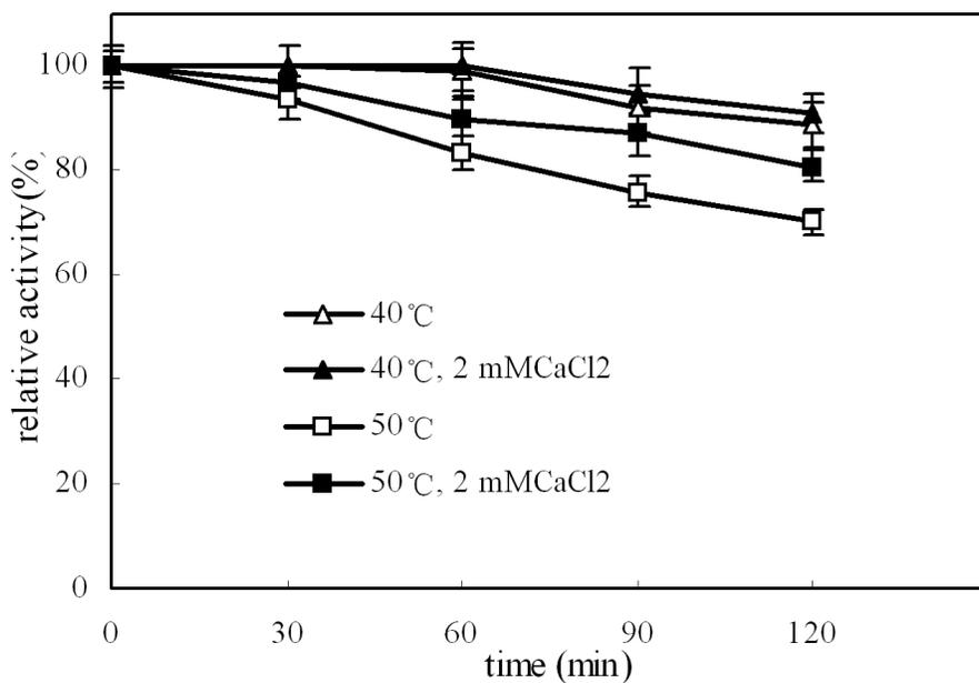
**Figure 10.** Effect of temperature on thermal stability of protease TC4. The enzyme was preincubated in the absence or presence of 2 mM CaCl<sub>2</sub>. Remaining activity was determined at intervals under the optimal conditions. The original activity before preincubation was taken as 100%.
