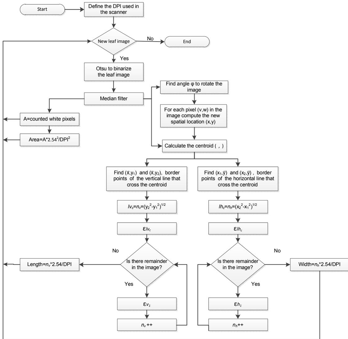
Figure 3. Flow diagram of SIM's image processing.
