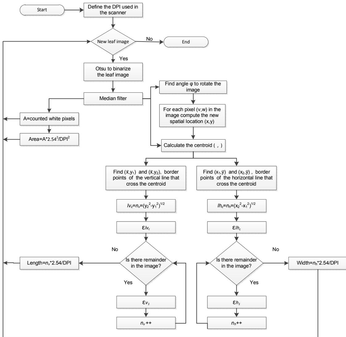
Figure 3. Flow diagram of SIM's image processing.
