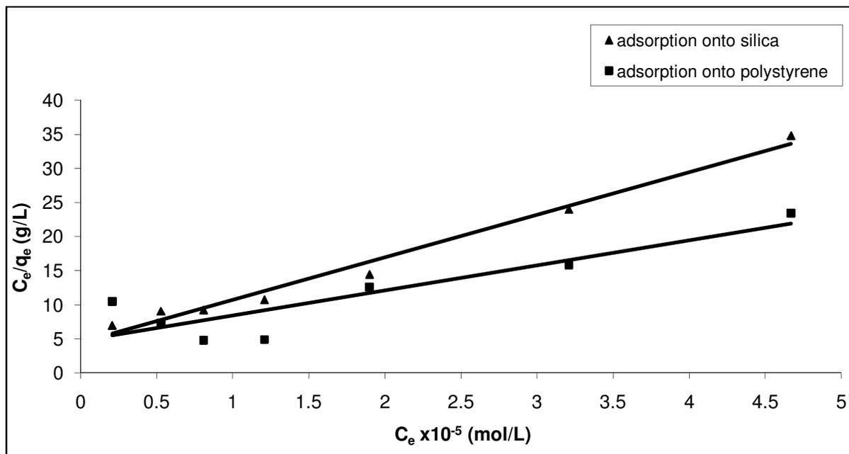
**Figure 5.** Langmuir isotherm plot of  $C_e/q_e$  against  $C_e$  for adsorption of lysozyme onto the surfaces.
