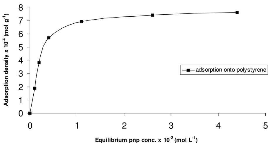
**Figure 3.** The variation of adsorption capacity (mol g<sup>-1</sup> polystyrene) with equilibrium paranitrophenol concentrations.
