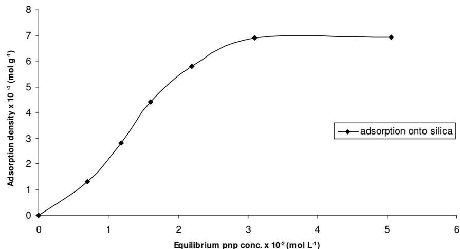
**Figure 2.** The variation of adsorption capacity (mol g<sup>-1</sup> silica) with equilibrium paranitrophenol concentrations.
