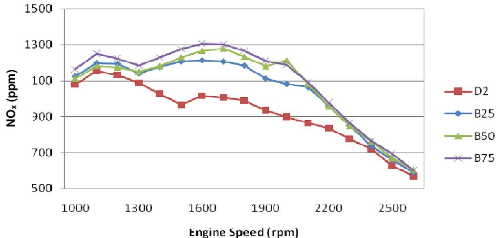
Figure 4. NO<sub>x</sub> emissions of the biodiesel and diesel fuels.
