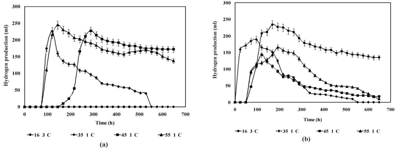
**Figure 3.** Hydrogen production (ml) a) initial pH 4.0 and b) initial pH 11.3; initial concentration 21.1 g/l COD at different temperatures ( $16 \pm 3$ ,  $35 \pm 1^\circ\text{C}$ ,  $45 \pm 1^\circ\text{C}$  and  $55 \pm 1^\circ\text{C}$ ).
