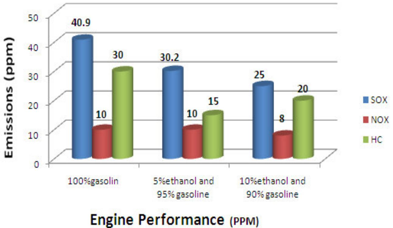
Figure 7. Engine emission of Hc. Nox. Sox.
