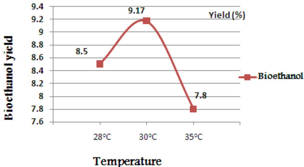
Figure 2. The bioethanol yield in different temperature.
