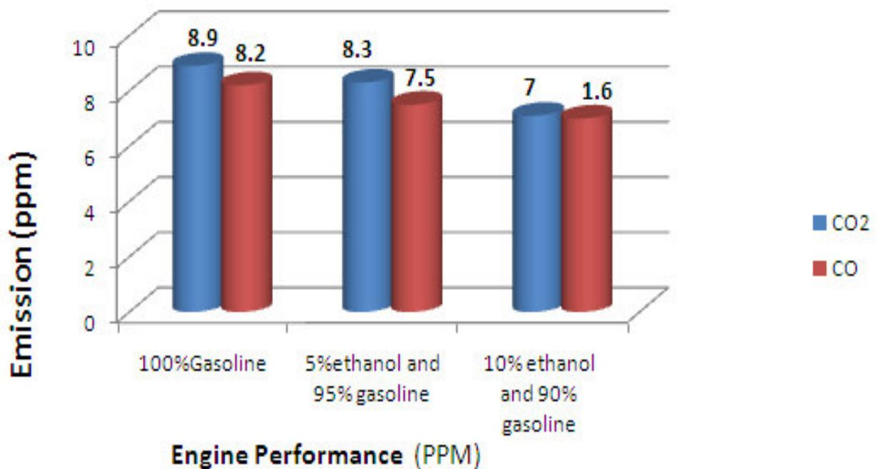
Figure 8. Engine emission of Co. Co<sub>2</sub>.
