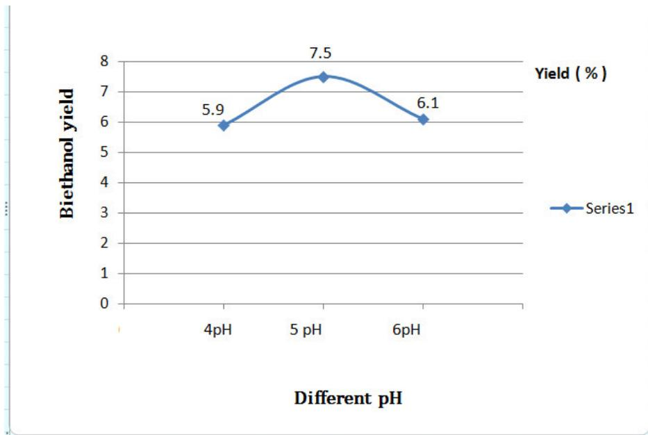
Figure 1. The bioethanol yield in different pH parameters.
