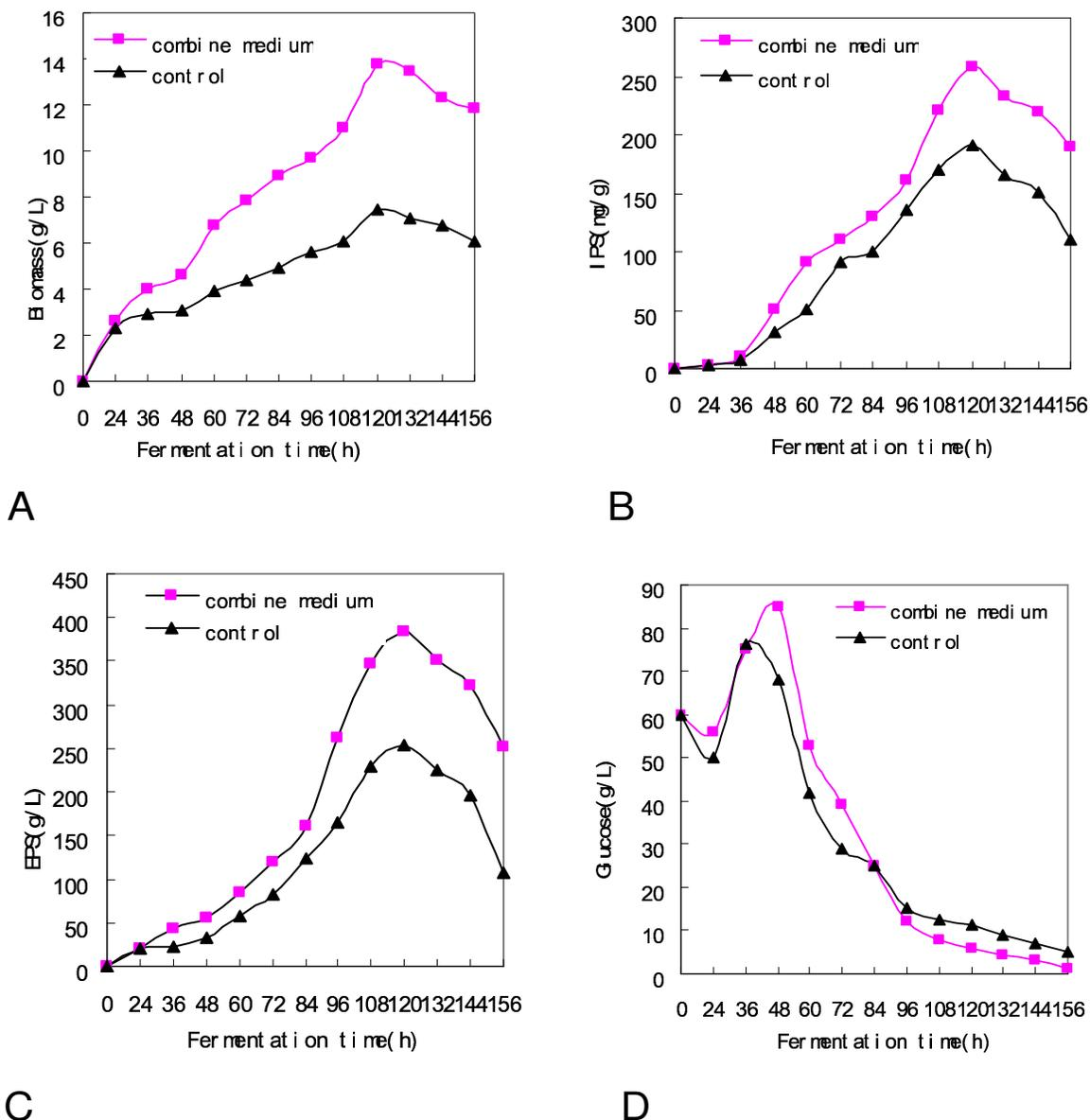
**Figure 3.** The dynamics of biomass, polysaccharide accumulation and reduce glucose in the optimum growth medium in shake flask (cultures medium components: peptone, 10; glucose, 60;  $\text{KH}_2\text{PO}_4 \cdot \text{H}_2\text{O}$ , 1.5; vitamin B1, 0.01;  $\text{FeSO}_4$ , 50 ppm;  $\text{NaSeSO}_3$ , 25 ppm;  $\text{ZnSO}_4$ , 75 ppm; temperature: 30°C; rotates: 150 r/min; inoculum: 10%; pH: natural).
