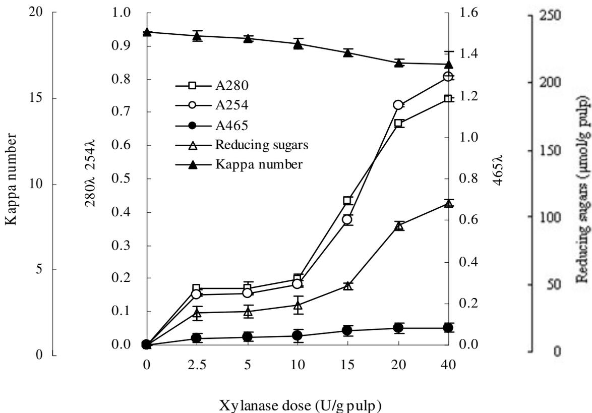
**Figure 8.** Optimization of xylanase dose for biobleaching of pulp. These experiments were performed at pH 7.0, temperature 50°C, at a retention time of 60 min and a pulp consistency of 5%. Symbols: open square, A280; open circle, A254; closed circle, A465; open triangle, reducing sugars; closed triangle, Kappa number.
