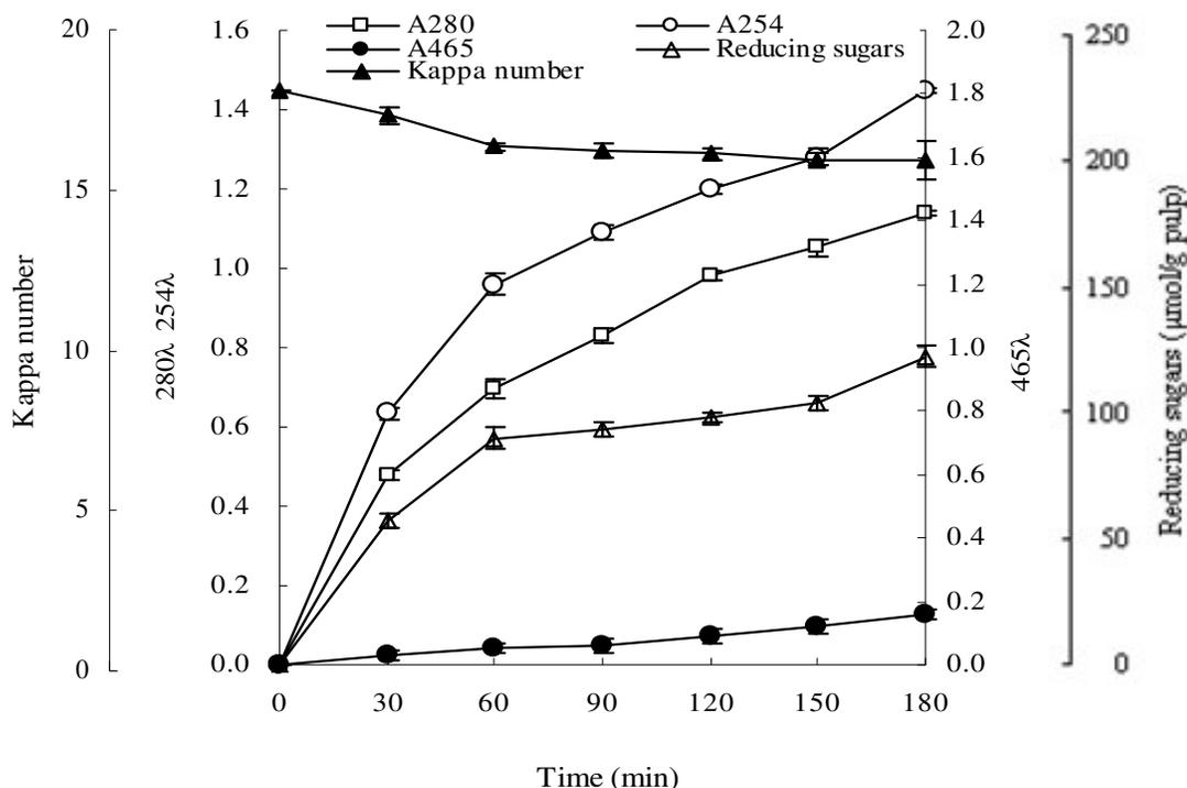
**Figure 9.** Optimization of retention time for biobleaching of pulp. These experiments were performed at pH 7.0, temperature 50°C and a pulp consistency of 5%. Symbols: open square, A280; open circle, A254; closed circle, A465; open triangle, reducing sugars; closed triangle, Kappa number.
