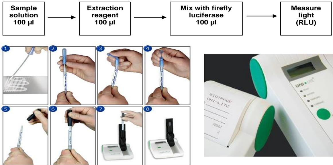
Figure 1. Biotrace uni- lite sampling procedure, hygienia.
