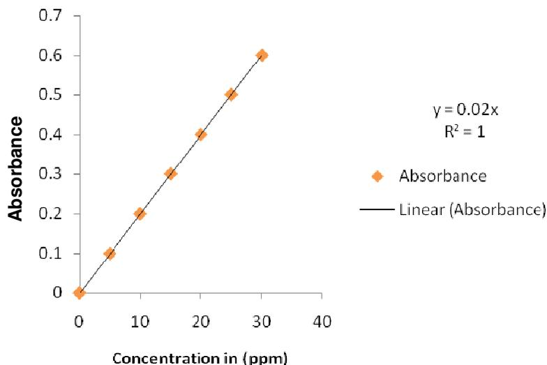
Figure 2. Calibration curve using oxine chloroform solution.
