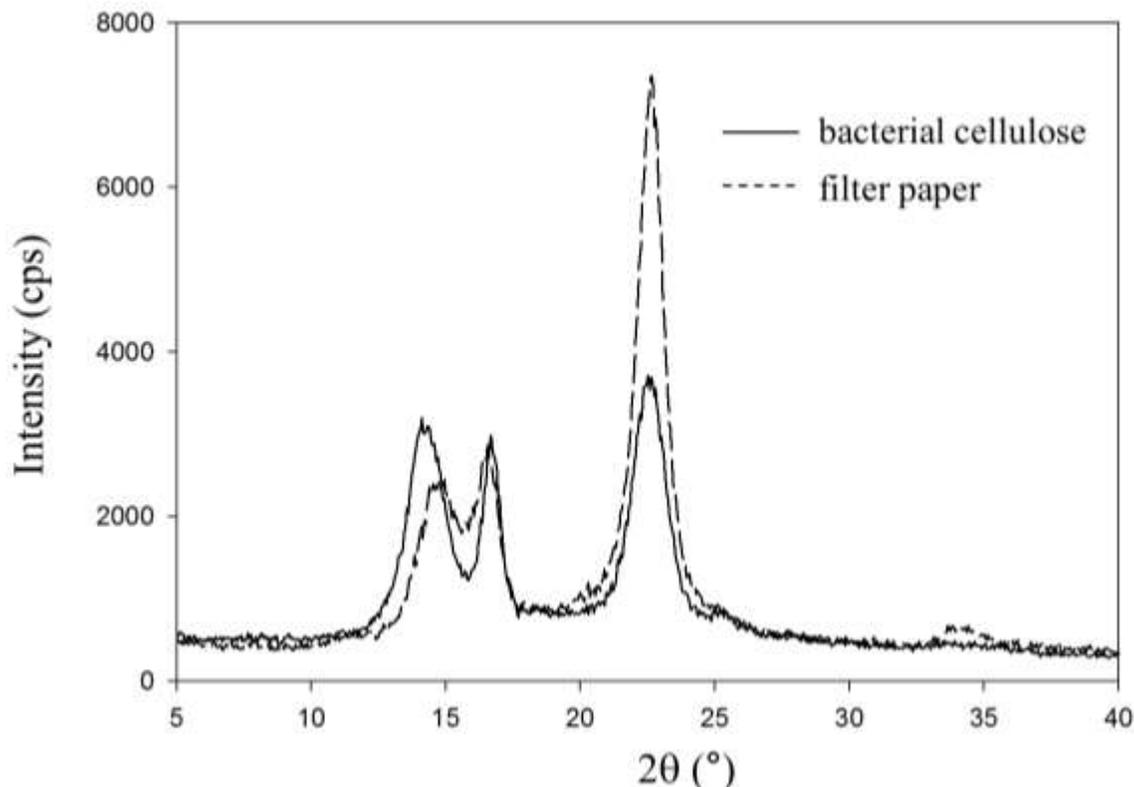
**Figure 4.** X-Ray diffraction patterns obtained from filter paper and BC produced by *Gluconacetobacter* sp. RKY5.
