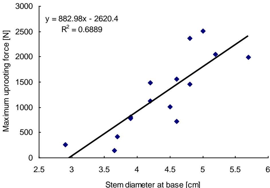
**Figure 5.** The relation between the maximum uprooting force and the stem diameter at base of *S. alba var. tristis*.
