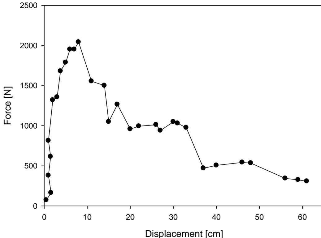
**Figure 1.** A typical uprooting–displacement curve for *S. alba var. tristis*.
