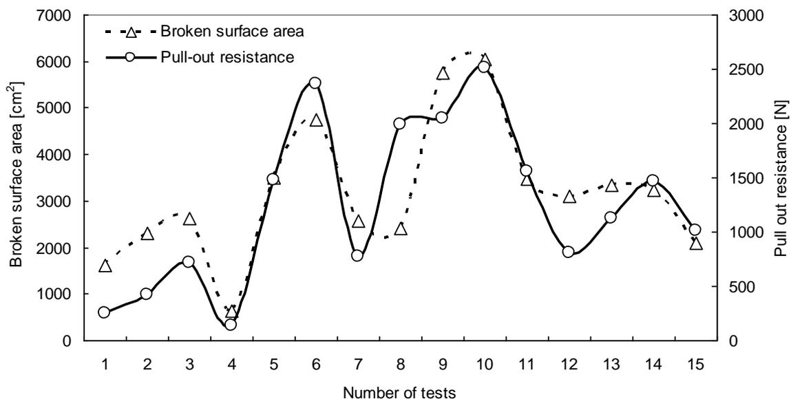
**Figure 6.** Uprooting resistance with broken surface area during the pull-out test.
