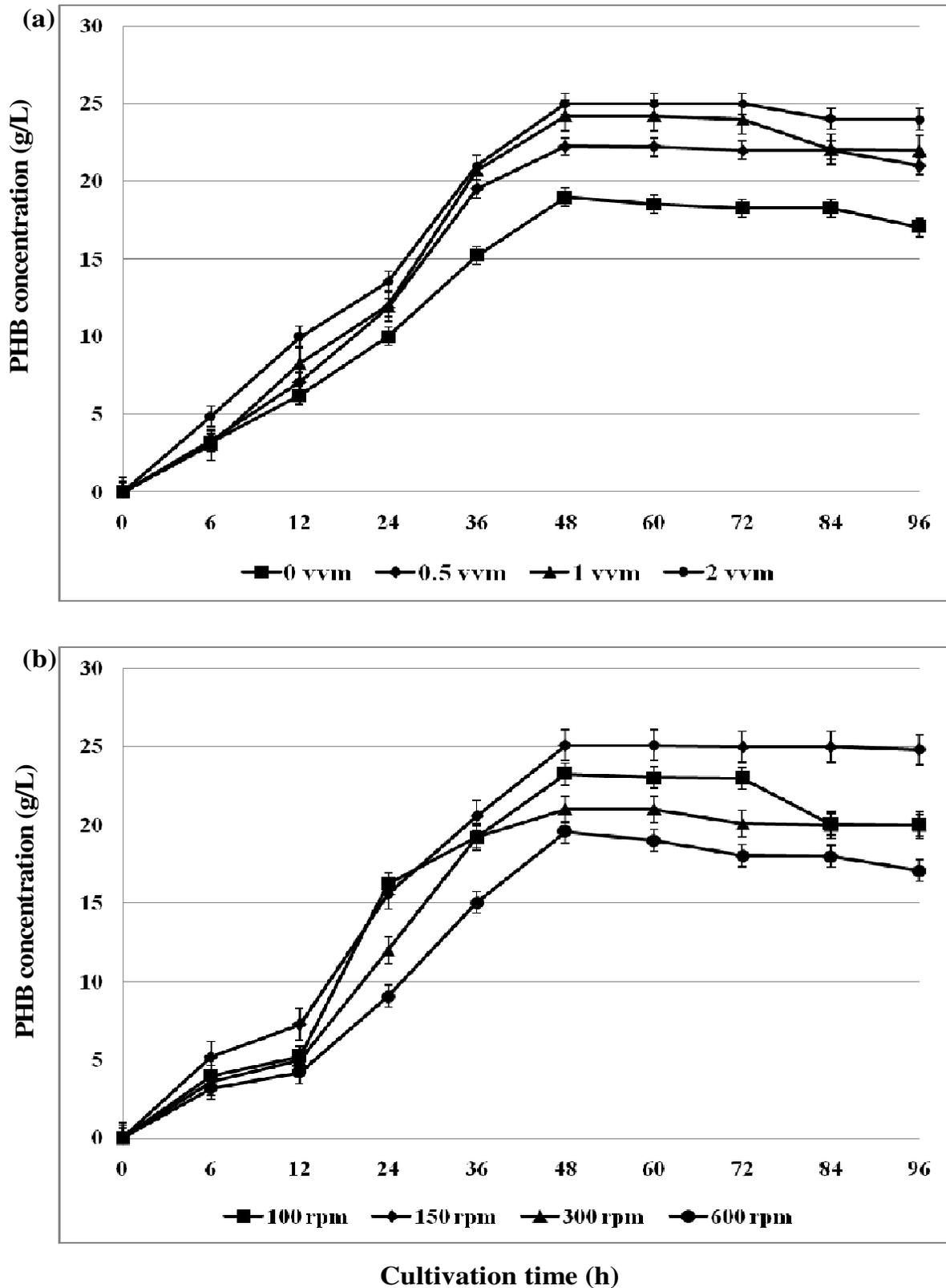
**Figure 2.** Effect of aeration rate (a) and agitation speed (b) on PHB content from *Cupriavidus necator* TISTR 1095 cultured in glycerol-containing medium consisting of 60 g/L glycerol, 1.32 g/L  $(\text{NH}_4)_2\text{SO}_4$  and 2 g/L trace element at 30°C under pH control at 6.8.
