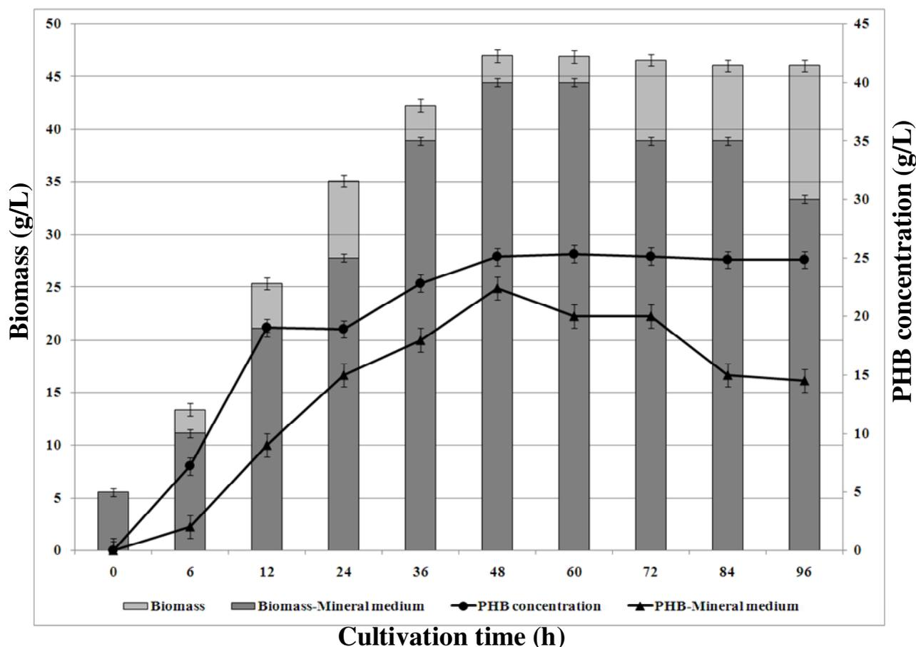
**Figure 3.** Growth (■, □) and PHB accumulation (●, ▲) of *Cupriavidus necator* TISTR 1095 on optimal medium containing glycerol (carbon source), 60 g/L;  $(\text{NH}_4)_2\text{SO}_4$  (nitrogen source), 1.32 g/L and trace element 2.00 g/L at 30°C, under controlled aeration rate (2 vvm), agitation speed (150 rpm), pH (6.8) conditions compared with mineral medium, respectively.
