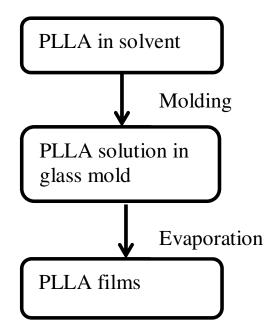
Figure 2. Schematic diagram of PLLA film fabrication.
