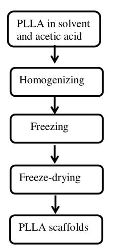
Figure 1. Schematic diagram of PLLA scaffold production.
