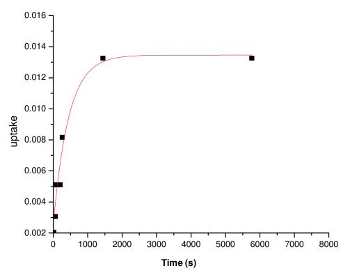
Figure 6. Water uptake profile of PLLA film.
