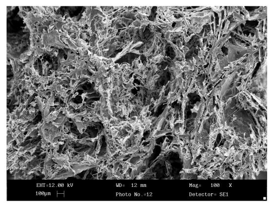
Figure 3. Scanning electron micrograph (SEM) of PLLA scaffold.
