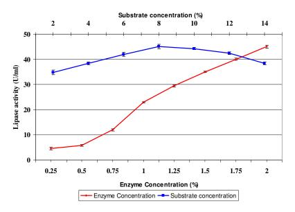
**Figure 4.** Effect of substrate (olive oil) and enzyme concentrations on lipase activity produced by *M. geophillus*. The enzyme was measured at pH 6.5, and  $35 \,^\circ$ C.
