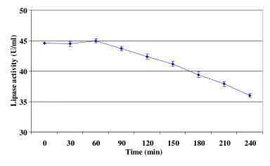
**Figure 2.** Effect of time on lipase activity produced by *M. geophillus*. The enzyme was measured at pH 6.5, and  $37 \,^{\circ}$ C.
